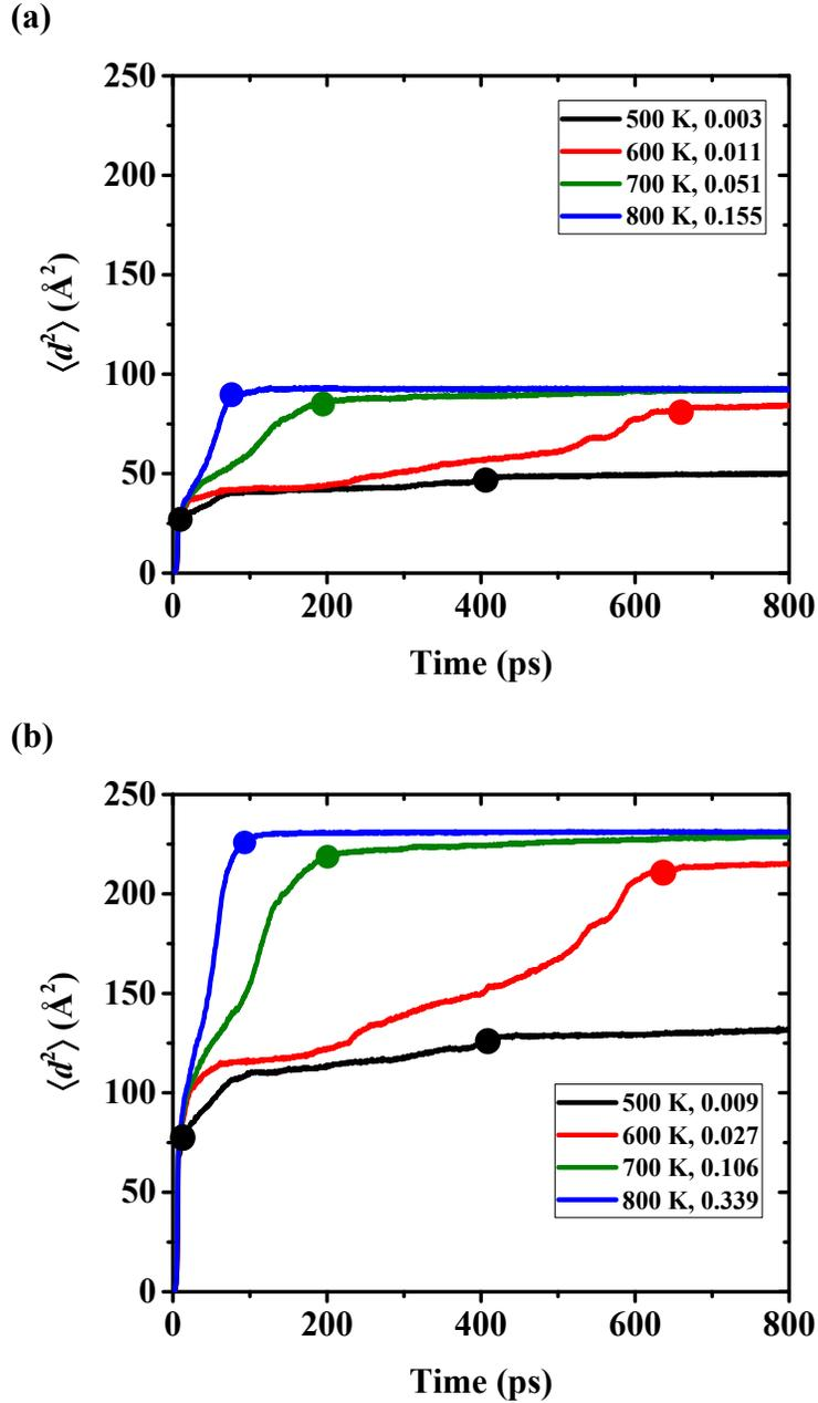
**Figure S4:** Mean square displacement ( $\langle d^2 \rangle$ ) of the (a) surface and (b) shell atoms during the sintering of multiple  $\text{Ag}_5\text{Cu}_{2.5}$  NPs. The self-diffusivity (in the unit of  $\text{\AA}^2/\text{ps}$ ) obtained by linear fitting is also shown after each  $T$ . The dots in each curve represent the starting and ending points, during which the  $\langle d^2 \rangle$  is used to calculate the self-diffusivity and activation energy.
