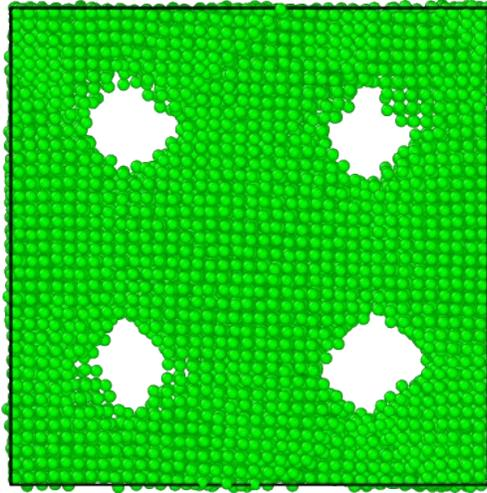
**Figure S3:** Final sintered structure of multiple  $\text{Ag}_5\text{Cu}_0$  NPs (pure Ag NPs) at 600 K. Pores are not eliminated at this  $T$ , while the pores do not survive in multiple CS NPs at 600 K, which proves that the interfacial atoms have higher mobility in CS NP and contribute to a higher densification.
