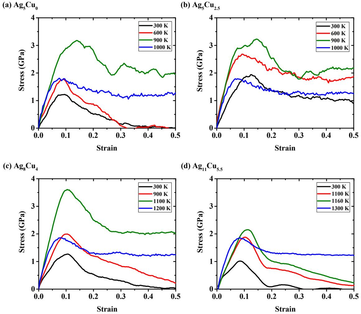
**Figure S5:** Stress-strain plots for structures sintered by multiple NPs (a)  $\text{Ag}_5\text{Cu}_0$ , (b)  $\text{Ag}_5\text{Cu}_{2.5}$ , (c)  $\text{Ag}_8\text{Cu}_4$ , and (d)  $\text{Ag}_{11}\text{Cu}_{5.5}$  at different  $T^s$ 's. Note that all tensile simulations are performed at 300 K, i.e., the final sintered structures are quenched to 300 K before executing the tensile simulations.
