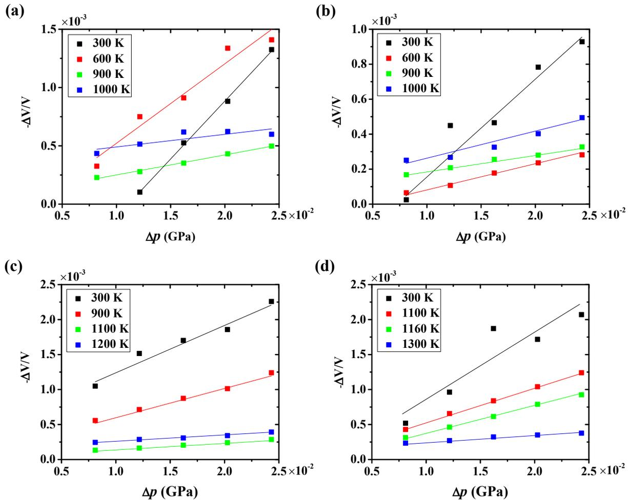
**Figure S7:** Plots of  $(-\Delta V/V_0 - \Delta p)$  of structures sintered by multiple NPs (a)  $\text{Ag}_5\text{Cu}_0$ , (b)  $\text{Ag}_5\text{Cu}_{2.5}$ , (c)  $\text{Ag}_8\text{Cu}_4$ , and (d)  $\text{Ag}_{11}\text{Cu}_{5.5}$  at different  $T$ 's. Isothermal compressibility is the slope of the linear fitting lines.
