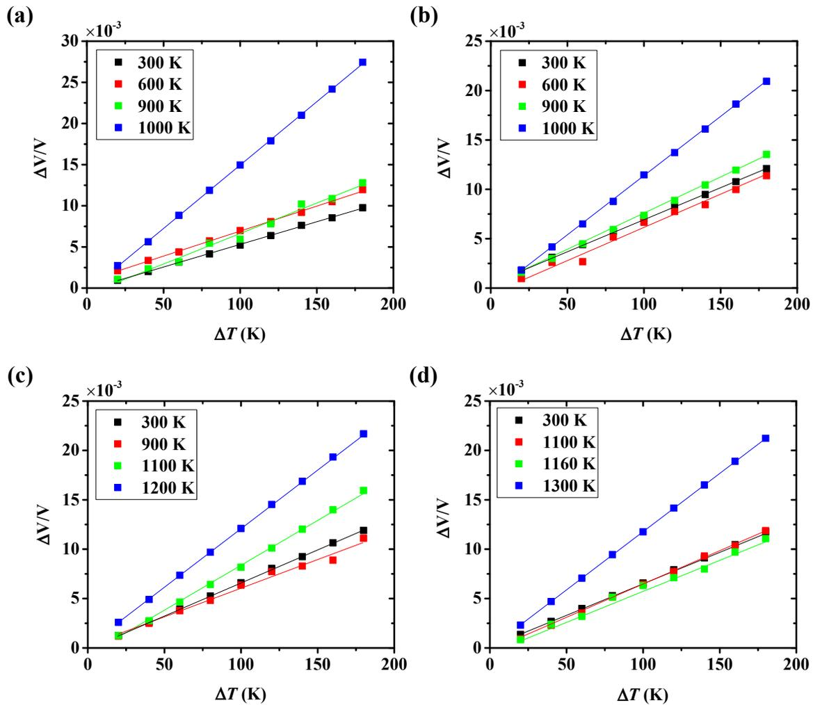
**Figure S8:** Plots of  $(\Delta V/V_0 - \Delta T)$  of structures sintered by multiple NPs (a)  $\text{Ag}_5\text{Cu}_0$ , (b)  $\text{Ag}_5\text{Cu}_{2.5}$ , (c)  $\text{Ag}_8\text{Cu}_4$ , and (d)  $\text{Ag}_{11}\text{Cu}_{5.5}$  at different  $T^s$ s. Coefficient of thermal expansion is the slope of the linear fitting lines.
