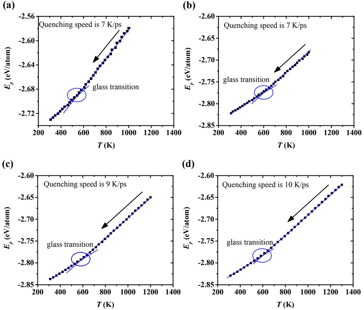
**Figure S6:** Potential energy ( $E_p$ ) evolution during the quenching process of the sintered structures of multiple NPs (a)  $\text{Ag}_5\text{Cu}_0$ , (b)  $\text{Ag}_5\text{Cu}_{2.5}$ , (c)  $\text{Ag}_8\text{Cu}_4$ , and (d)  $\text{Ag}_{11}\text{Cu}_{5.5}$ . No steep decrease of  $E_p$  is observed in these curves, indicating the formation of metallic glass after the quenching process.
