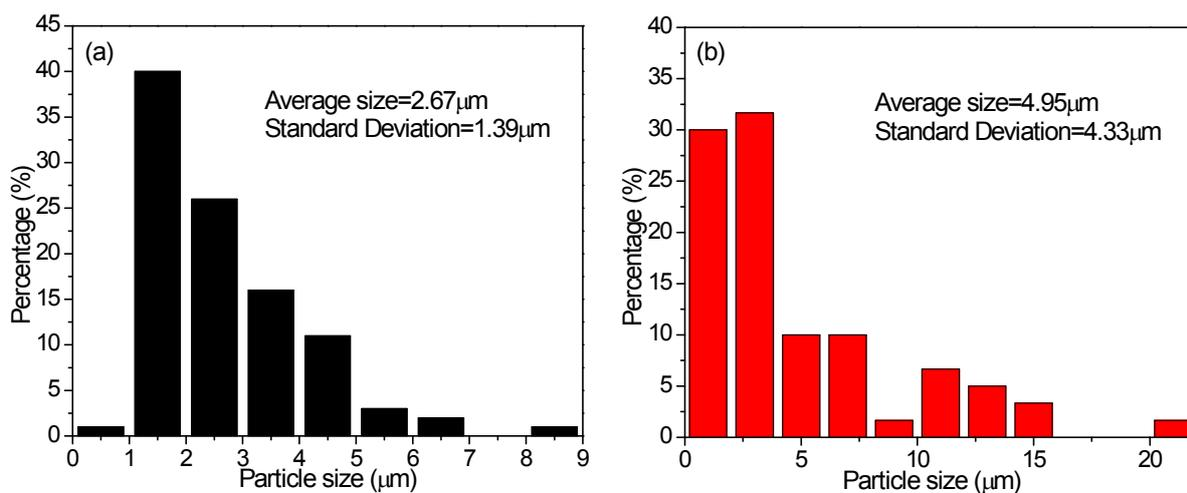
**Fig. S4** Histograms for particle size distribution of (a) OA-a and (b) OA-m in the PLLA melt. The particle size was measured by analysis software of POM.
