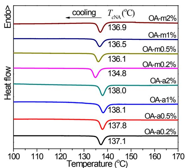
**Fig. S2** DSC thermograms of nonisothermal melt crystallization for PLLA/OA blends at the cooling rate of 1°C/min. Crystallization peak temperature ( $T_{cNA}$ ) is indicated below each curve.
