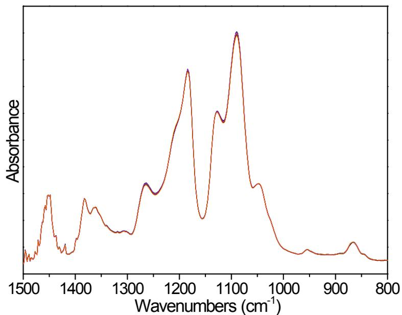
**Fig. S3** Time-resolved FTIR spectra of pure PLLA isothermally melt-crystallized at 140°C. The spectra are stacked every 15min.
