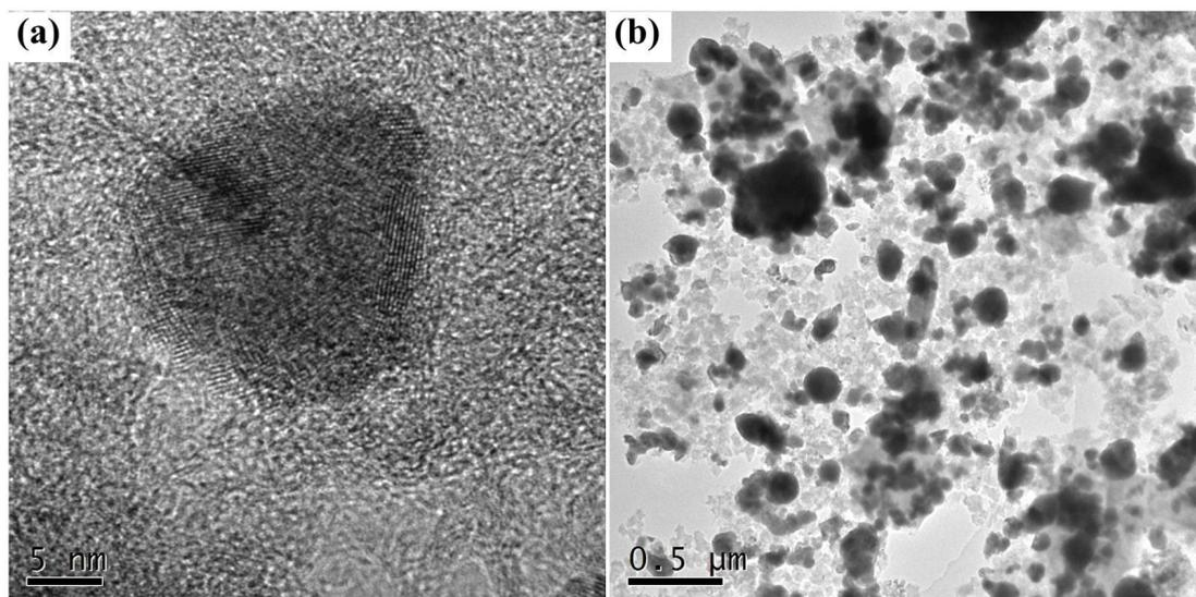
**Fig. S10** TEM image of SOC-3 after tenth cycle in the current density of 500 mA g<sup>-1</sup>.
