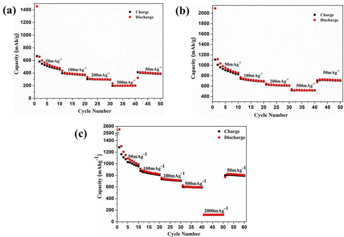
**Fig. S8** Rate performances of SOC-3 (a) from 50 to 2000 mA g<sup>-1</sup>, SOC-1 (a) and SOC-3 (b) electrodes from 50 to 500 mA g<sup>-1</sup> and SOC-3 (c) from 50 to 2000 mA g<sup>-1</sup>.
