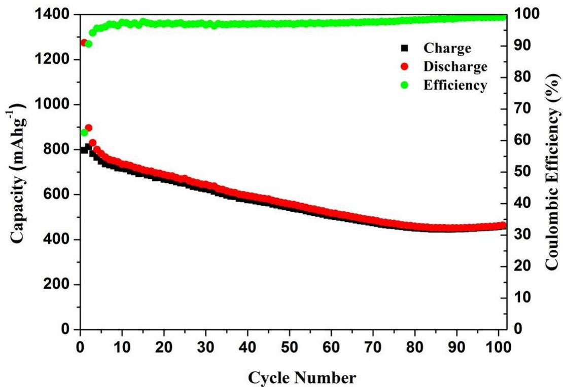
Fig. S9 Charge-discharge curve of the electrode made of SOC-3 at 500 mA g<sup>-1</sup>.
