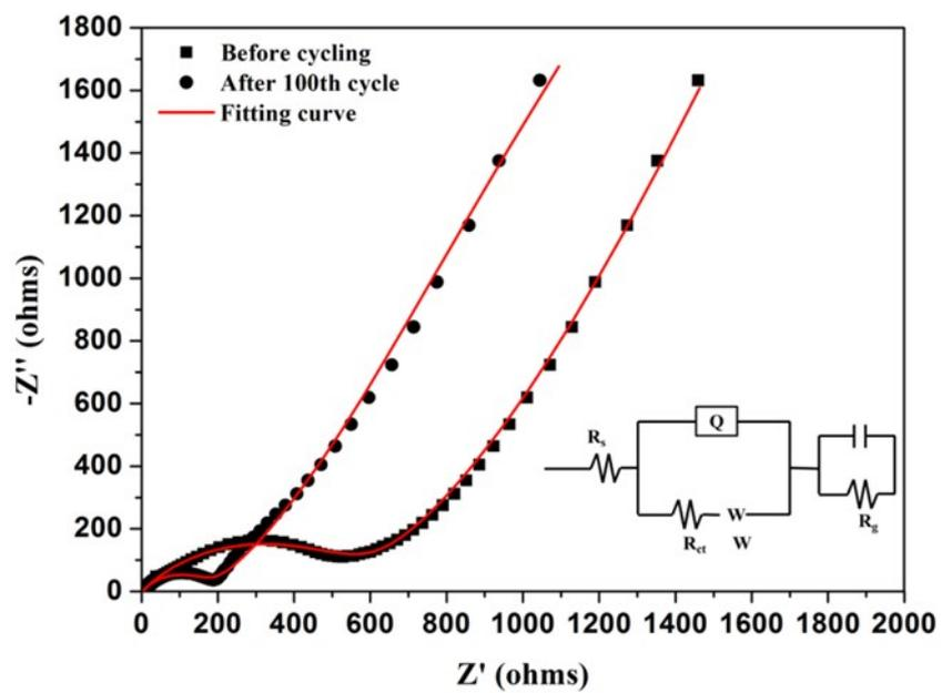
Fig. S11 The electrochemical impedance spectra of SOC-3.
