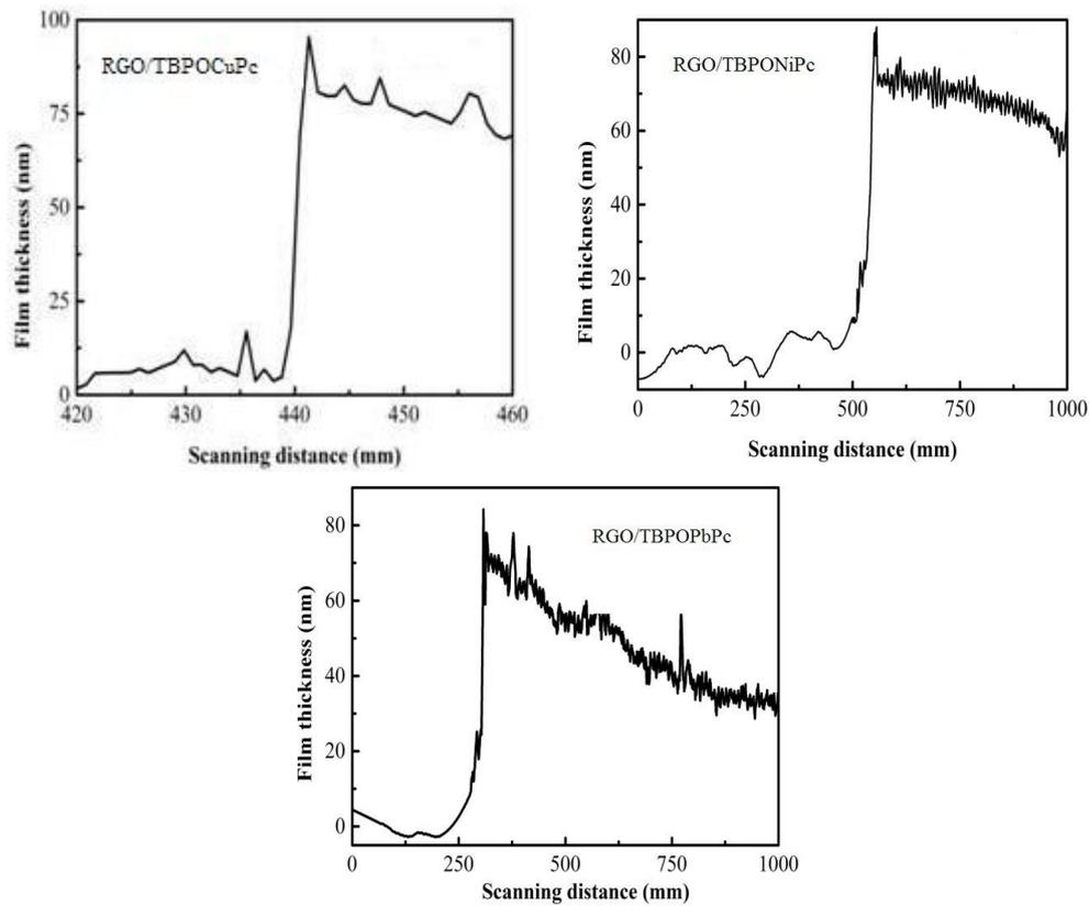
Fig. S2. Film thicknesses of RGO/TBPOMPc (M= Cu, Ni, Pb) placed on the electrodes.
