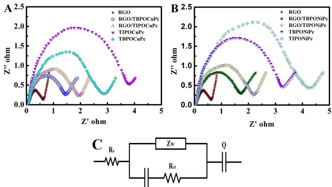
Fig.S12. EIS measurements of RGO, RGO/TIPOMPC, RGO/TBPOMPC, TIPOMPC and TBPOMPC (M= Cu and Ni) electrodes in 6 M KOH aqueous solution (A-B); (C) shows the corresponding electrical equivalent circuit.
