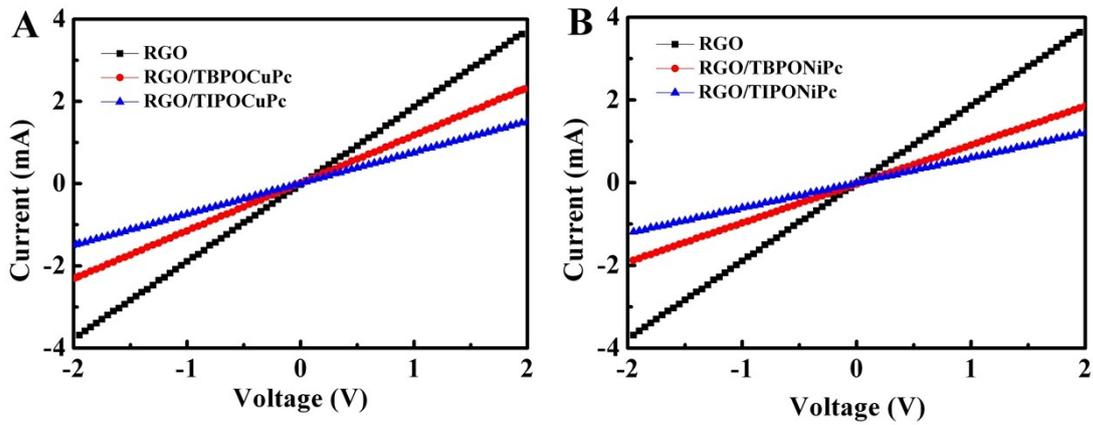
Fig. S11.  $I-V$  curves of RGO, RGO/TBPOMPc and RGO/TIPOMPc ( $M = Cu$  and  $Ni$ ) hybrids.
