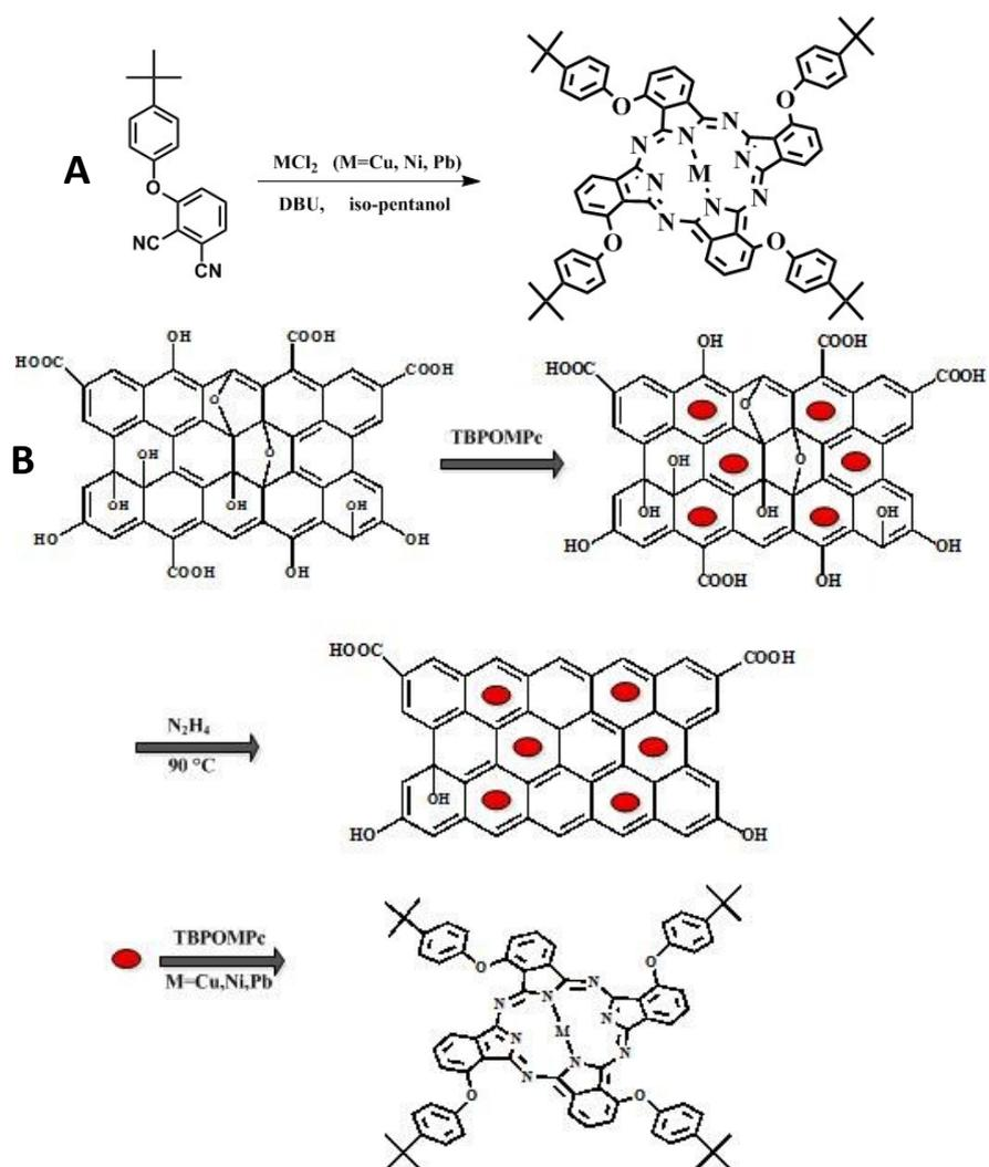
Fig. S1. The schematic interaction process for the preparation of (A) TBPOMPc and (B) RGO/TBPOMPc hybrids.
