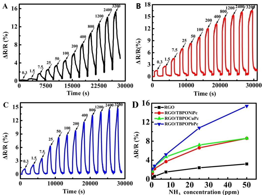
Fig. S7. Dynamic sensing response ( $\Delta R/R$ ) to different concentration of  $\text{NH}_3$  at room temperature.
