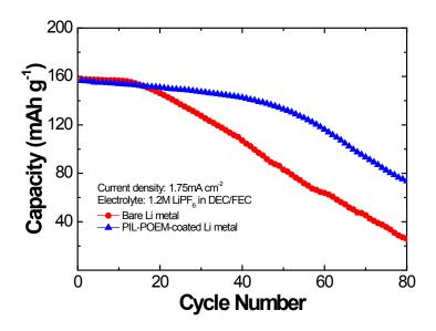
**Supplementary Fig. 1.** Cycling performance of coin-type cells. Discharging capacity vs. cycle number in carbonate for LCO/Li coin cells containing a bare Li metal anode and a PIL-POEM-coated Li metal anode.
