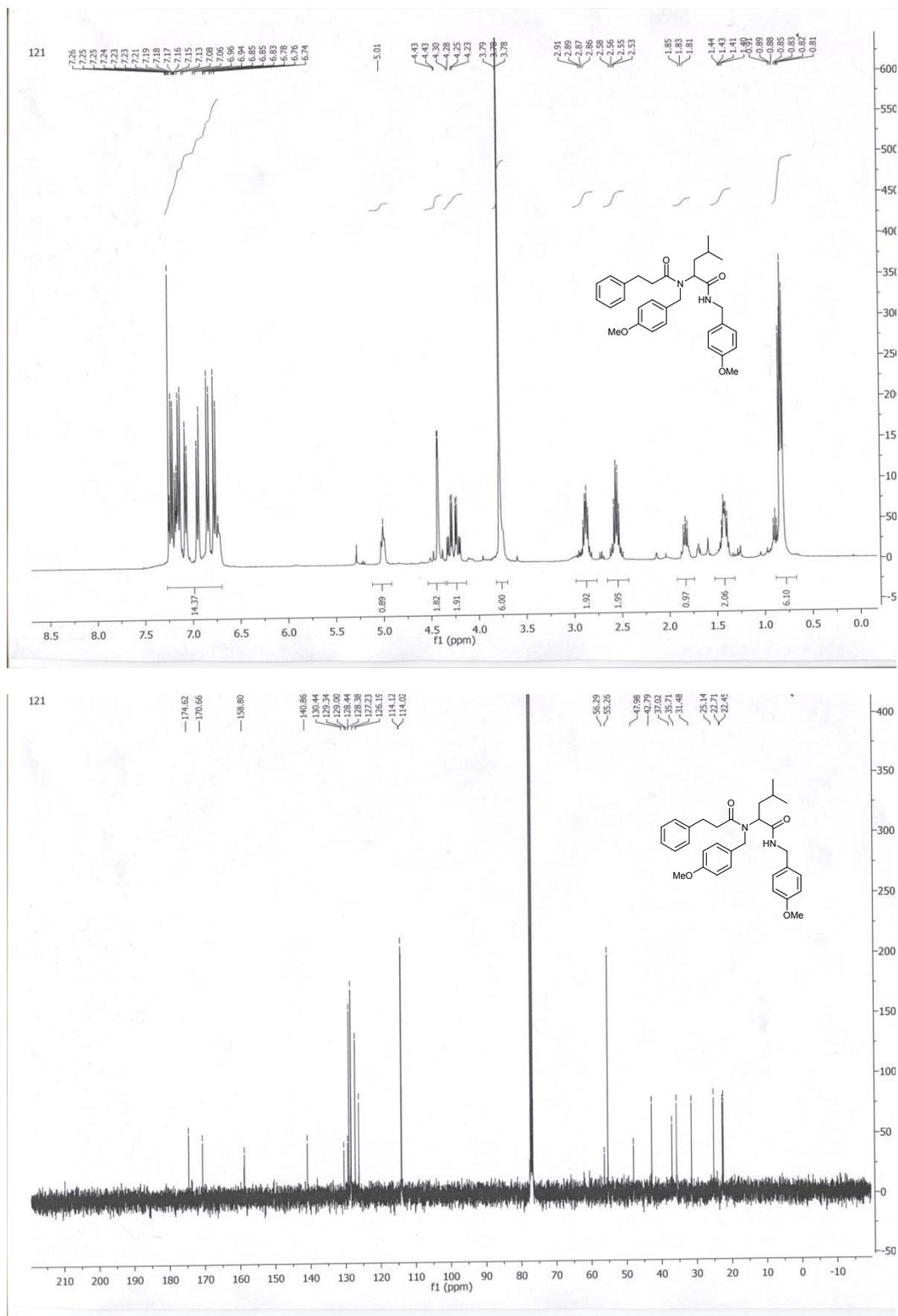
**Figure 11** <sup>1</sup>H NMR (above) and <sup>13</sup>C NMR (below) spectra of compound **5c** (400 MHz, CDCl<sub>3</sub>).
