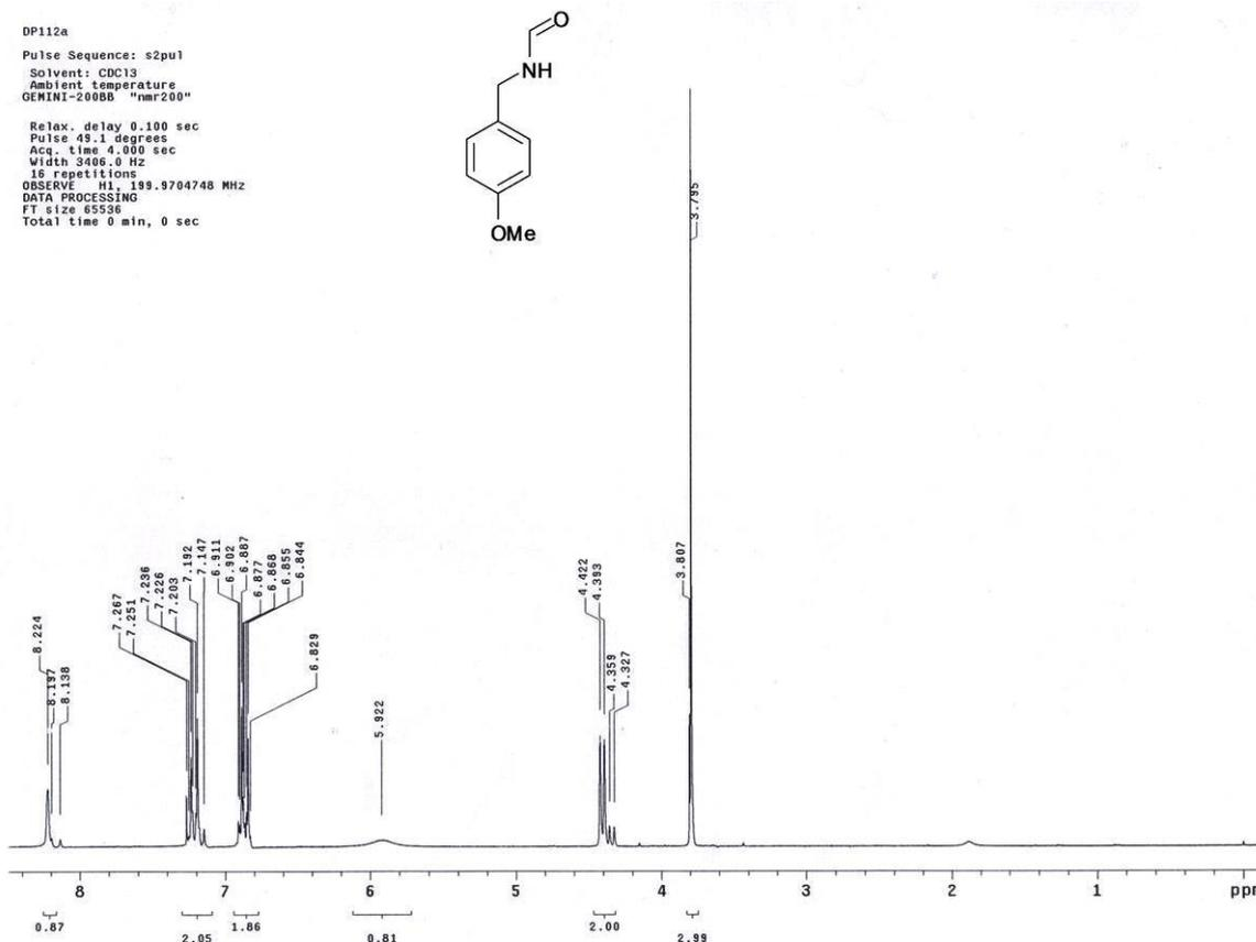
**Figure 1** <sup>1</sup>H NMR spectrum of *N*-(4-methoxybenzyl)formamide (200 MHz, CDCl<sub>3</sub>).
