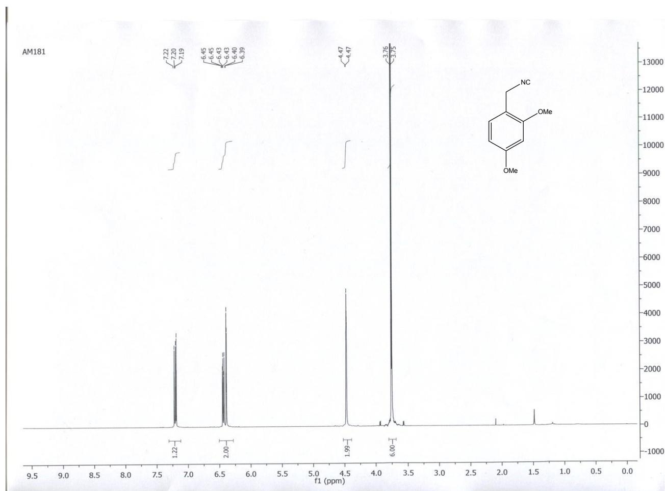
**Figure 6** <sup>1</sup>H NMR spectrum of 2,4-dimethoxybenzylisocyanide (400 MHz, CDCl<sub>3</sub>).
