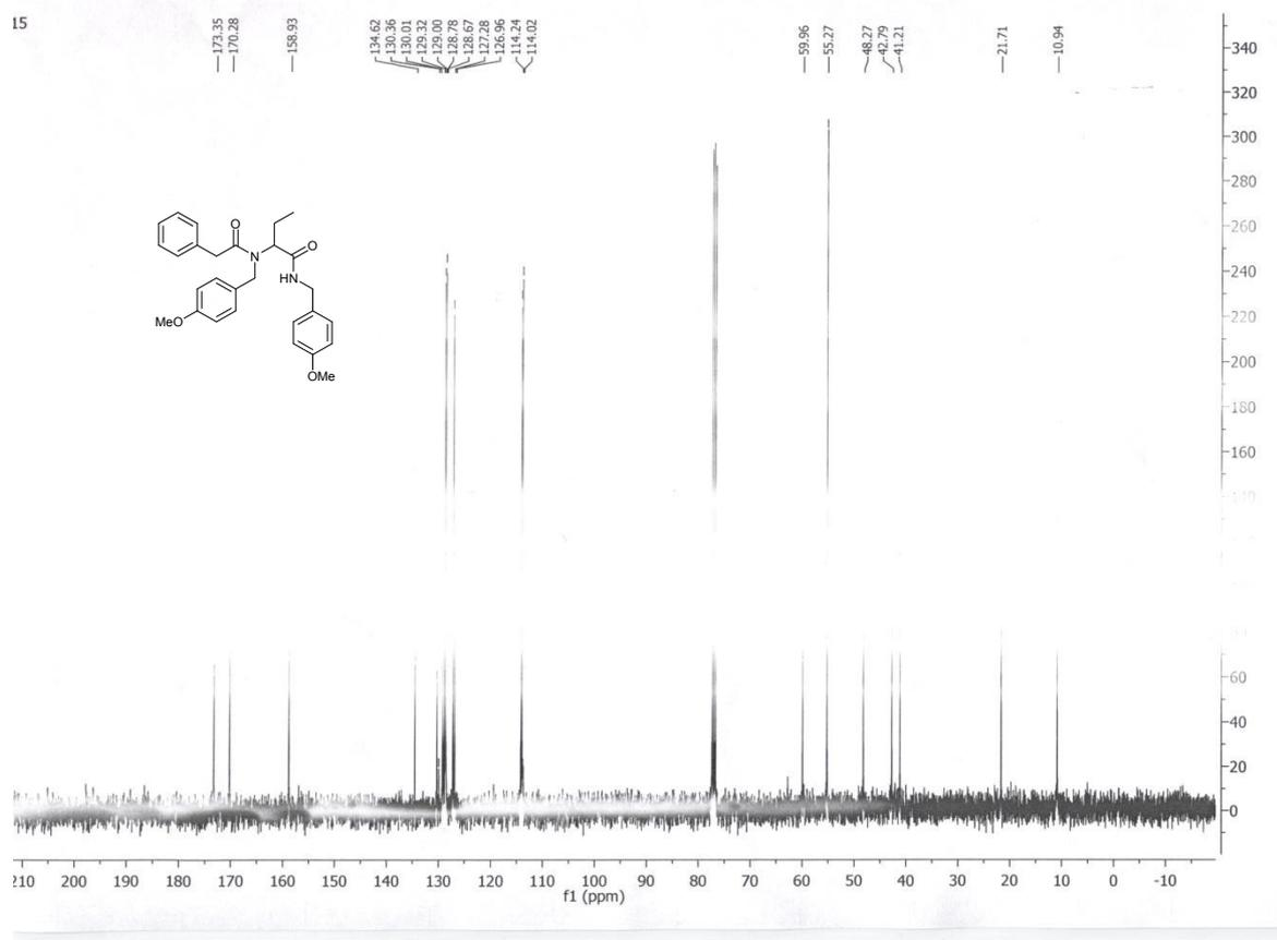
**Figure 15**  $^1\text{H}$  NMR (above) and  $^{13}\text{C}$  NMR (below) spectra of compound **5g** (400 MHz,  $\text{CDCl}_3$ ).
