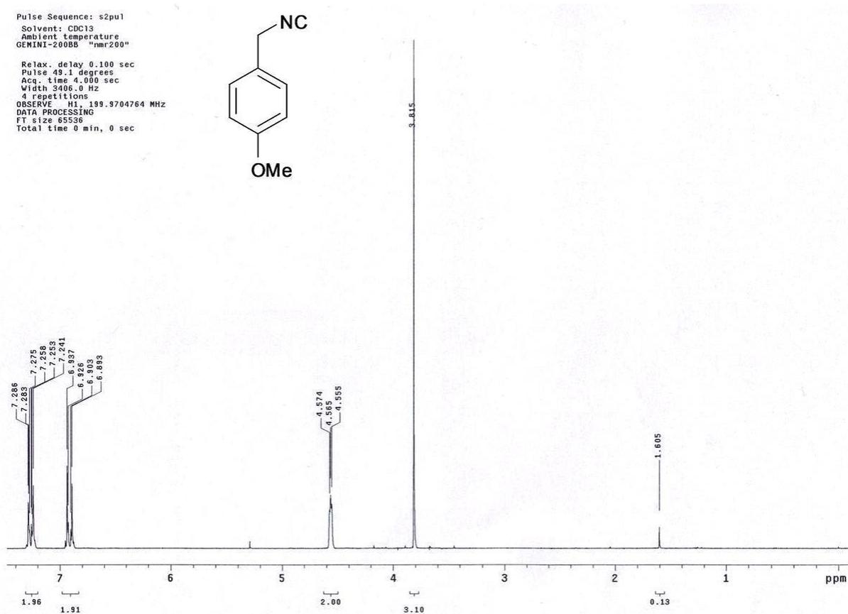
**Figure 2** <sup>1</sup>H NMR spectrum of compound **4a** (200 MHz, CDCl<sub>3</sub>).
