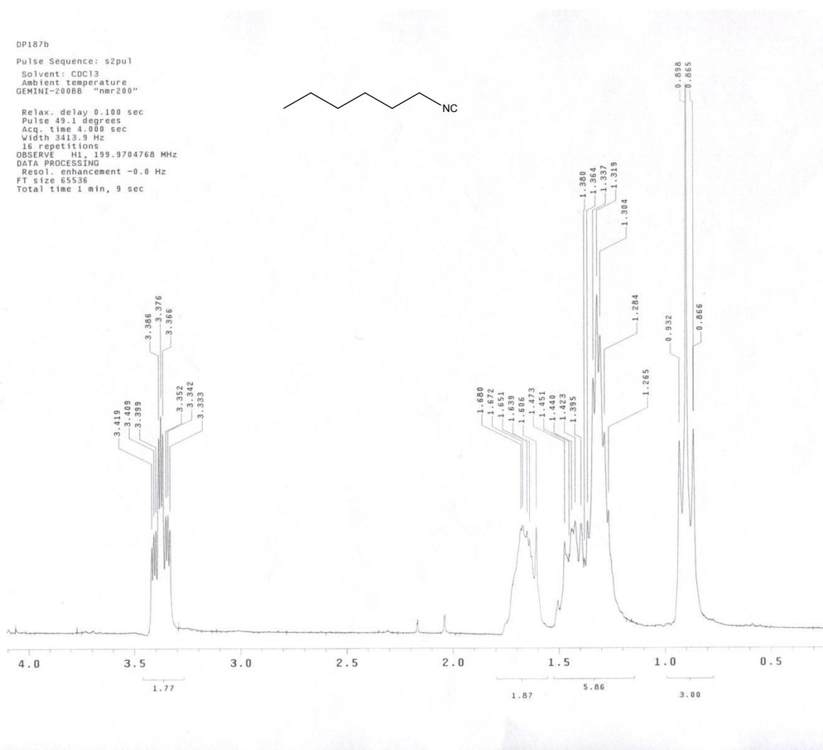
Figure 4 <sup>1</sup>H NMR spectrum of hexylisocyanide (200 MHz, CDCl<sub>3</sub>).
