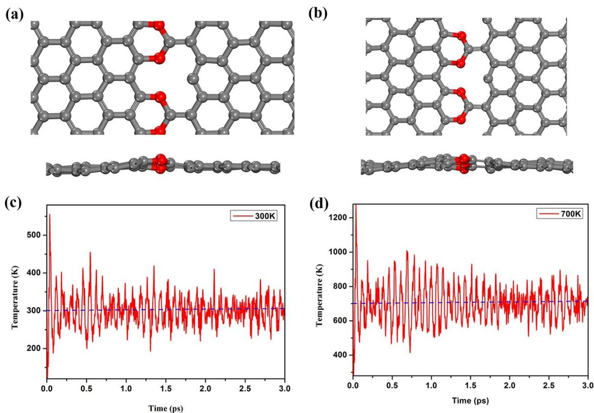
Fig. S3: Snapshots of the final configurations for each molecular dynamics simulation under (a) 300 and (b) 700 K (top and side views); The fluctuations of temperature as a function of the molecular dynamic simulation step at (c) 300K and (d) 700 K, respectively.
