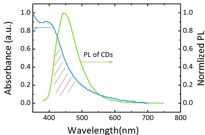
**Fig. S9.** The spectra overlap between CDs and PDA-FONSs.
