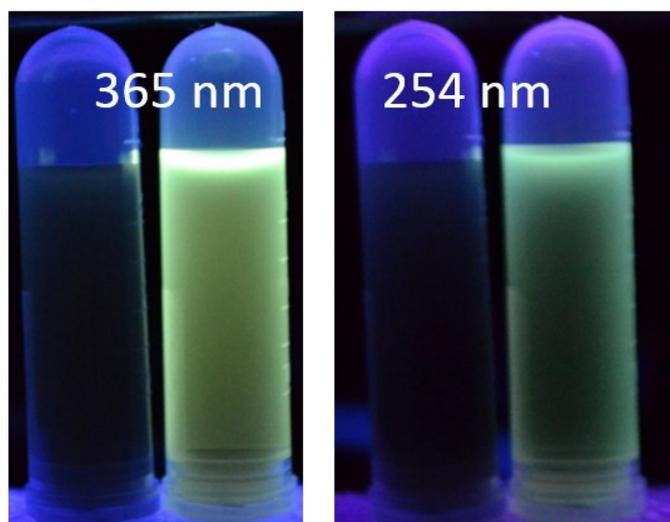
**Fig. S5.** The digital photos of PDA-FONs (left samples) and CDs-PDA-FONs (right samples) under UV lamp excited by 365 nm and 254 nm, respectively.
