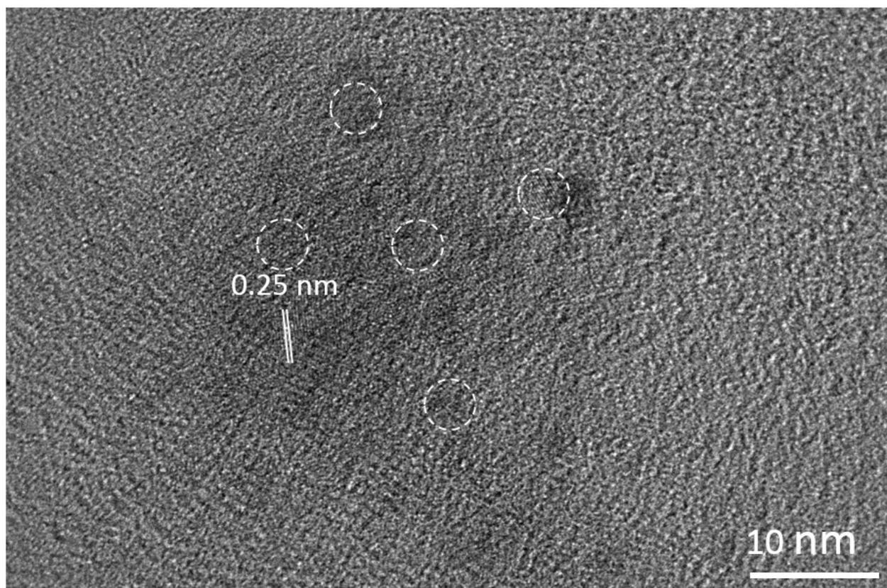
**Fig. S3** The High resolution TEM images of prepared CDs-PDA-FONs. The white circle was the inside CDs.
