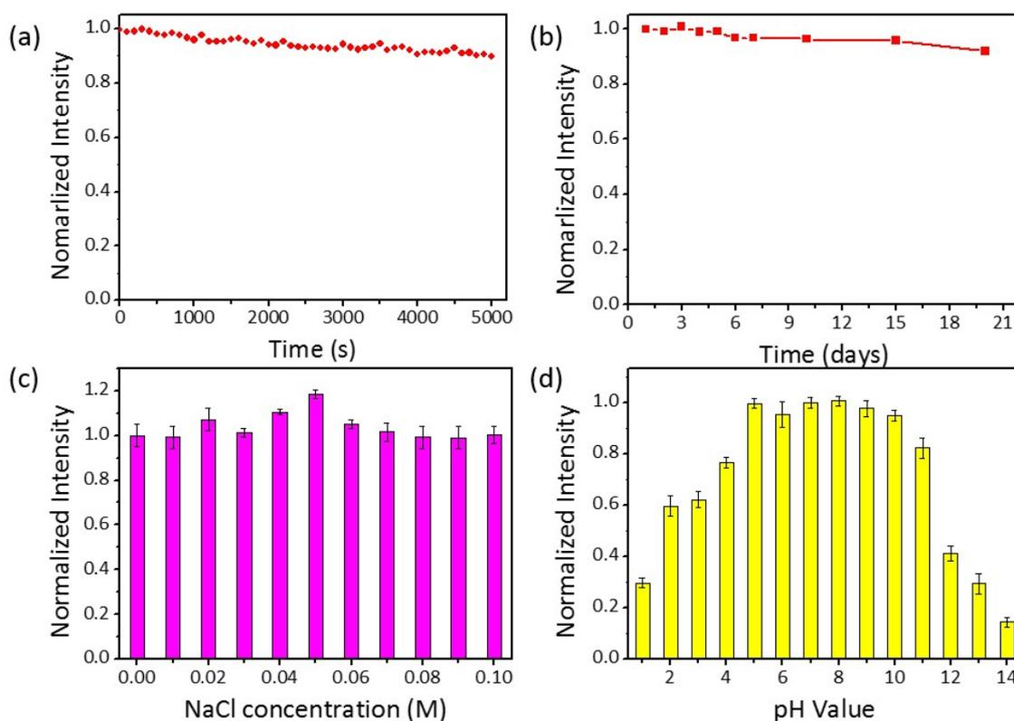
**Fig. S6.** The stability of as-prepared CDs-PDA-FONs. (a) Photostability which measured by continuous Xenon lamp radiation (50 W). (b) Storage stability in dark and  $-4^{\circ}\text{C}$ . The influence on fluorescence of CDs-PDA-FONs of concentration of NaCl (c) and pH value (d).
