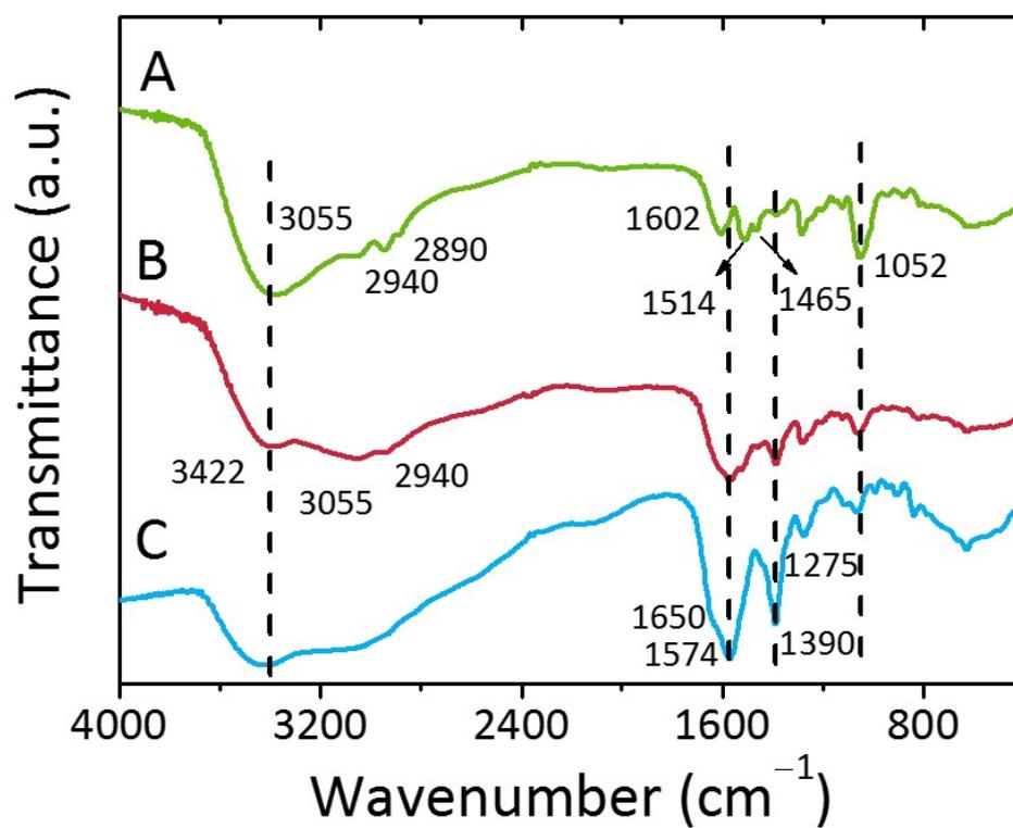
**Fig. S4** The FT-IR spectra of (A) CDs, (B) CDs-PDA-FONs and (C) PDA-FONs, respectively.
