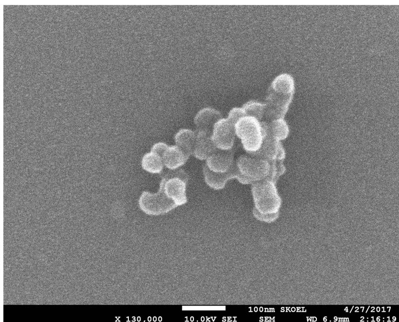
**Fig. S1** The SEM image of prepared CDs-PDA-FONs (measured in silicon slice).
