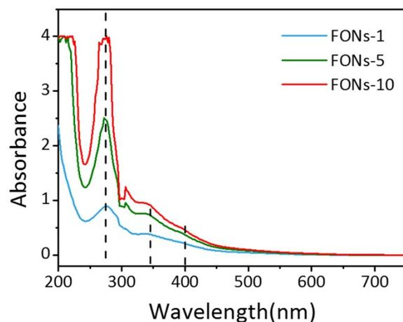
**Fig. S7.** The absorption spectra of different FONSs prepared at different reaction time for 1 h, 5 h, and 10h, respectively.
