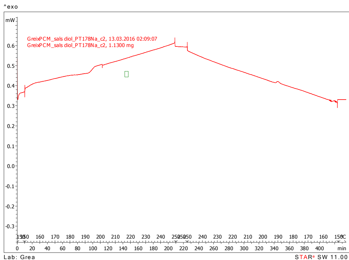
Figure 25. DSC response of sodium DHSA salt, 2 nd cycle.
