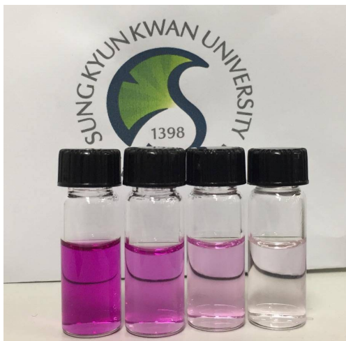
Fig. S3 Cr(VI) reduction to Cr(III) at 30 min after illumination using 1.1:1 SnS (with doped condition).
