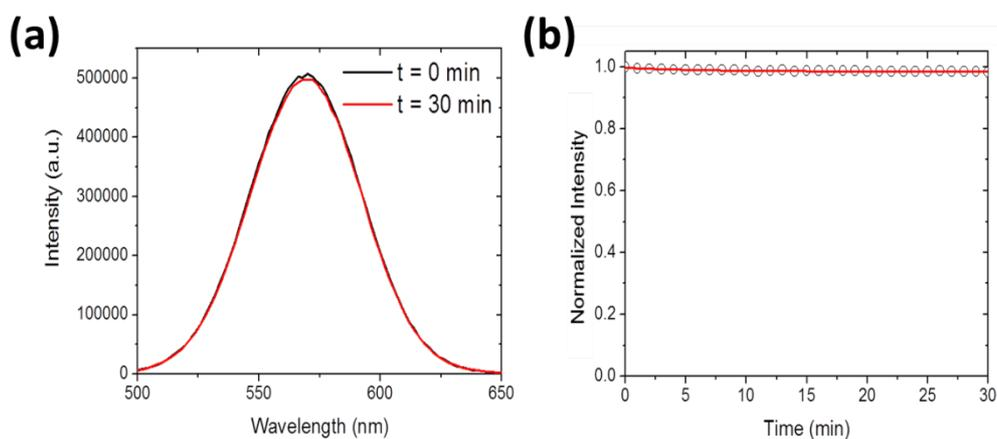
**Figure S4. Effect of  $\text{NaCl}$  on CdTe 580 emission.** (a) Normalized variation in fluorescence emission spectra of 25 nM CdTe 580 before ( $t = 0$  min) and after ( $t = 30$  min) injection of 120  $\mu\text{M}$   $\text{NaCl}$  at pH 8 with  $\lambda_{\text{exc}} = 400$  nm. (b) The corresponding normalized variation in fluorescence intensity across the entire 30 minute time window.
