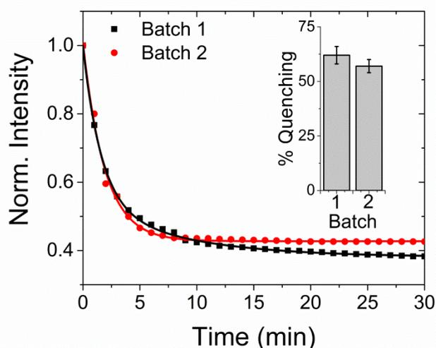
**Figure S2.** CdTe 580 quenching trajectories induced by  $Gd^{3+}$  display negligible batch-to-batch variation. Normalised variation in the fluorescence intensity of 25 nM CdTe 580 from two separate batches (red and black) as a function of time in the presence 10  $\mu M$   $Gd(NO_3)_3 \cdot 6H_2O$  in 20 mM Tris-HCl, pH 8 buffer. Inset: bar chart summarizing the quenching magnitude exhibited by two separated CdTe 580 batches after addition of 10  $\mu M$   $Gd^{3+}$  at  $t=30$  minutes.
