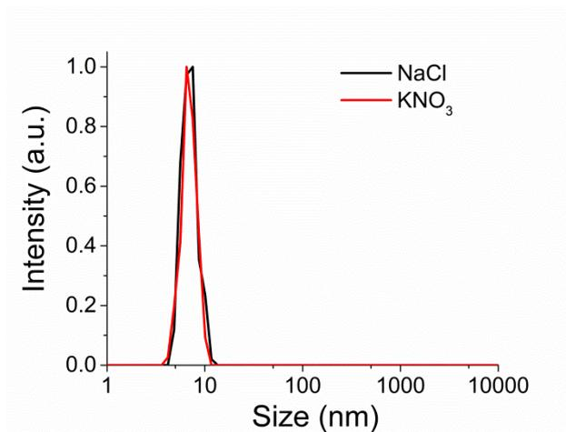
**Figure S5.** DLS size distributions of CdTe 580 QDs at  $t=30$  minutes, after injection of  $120 \mu\text{M}$  NaCl (black) and  $120 \mu\text{M}$   $\text{KNO}_3$  (red) at pH 8.
