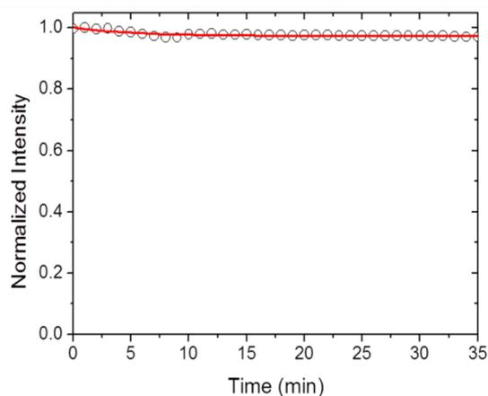
**Figure S3. Effect of  $\text{KNO}_3$  on CdTe 580 emission.** (a) Normalized variation in fluorescence emission intensity of 25 nM CdTe 580 after injection of 120  $\mu\text{M}$   $\text{KNO}_3$  at pH 8.  $\lambda_{\text{exc}} = 400$  nm.
