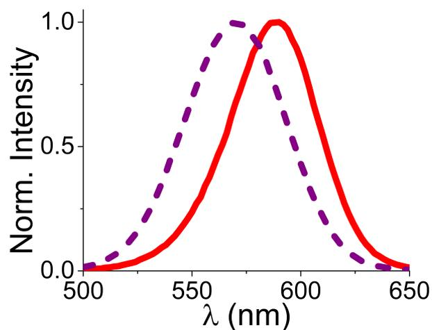
**Figure S1.** Normalized variation in CdTe 580 fluorescence emission spectra between the start ( $t=0$  min, dashed) and end ( $t=30$  min, solid) of the  $Gd^{3+}$  induced aggregation process.
