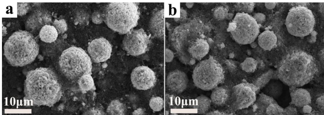
**Figure S3** SEM graphs of SD-NCA after different CV cycles: (a) the first cycle; (b) the third cycle
