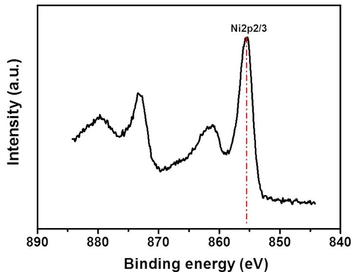
**Figure S1** The Ni 2p XPS spectrum of  $\text{LiNi}_{0.8}\text{Co}_{0.15}\text{Al}_{0.05}\text{O}_2$  powders.
