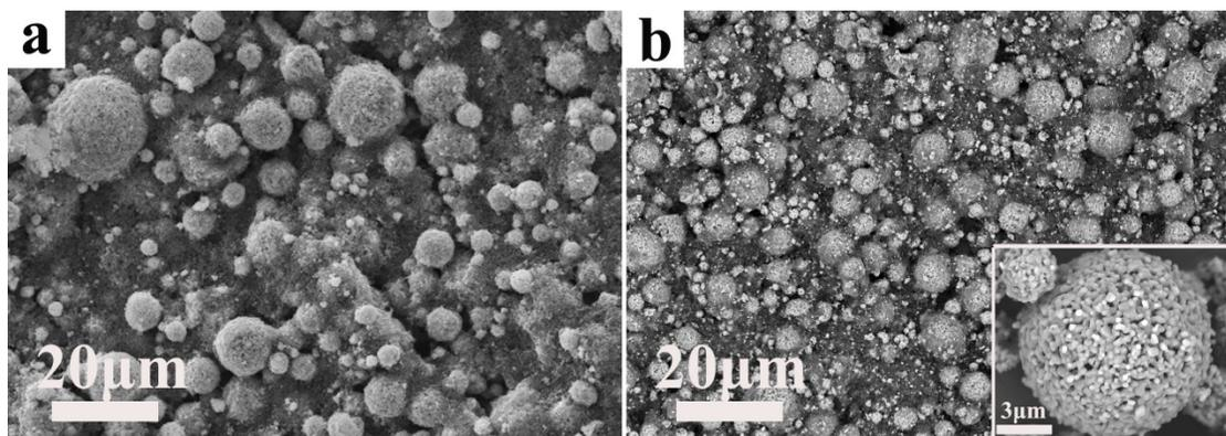
**Figure S4** SEM graphs of SD-NCA (a) before and (b) after 100 cycles at 1C.
