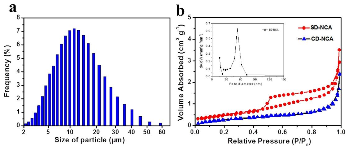
**Figure S2** (a) Particle size distribution of SD-LNCA; (b) nitrogen adsorption/desorption isotherms of CD-LNCA and SD-LNCA; (d) the insert illustrates the pore size distribution of SD-LNCA.
