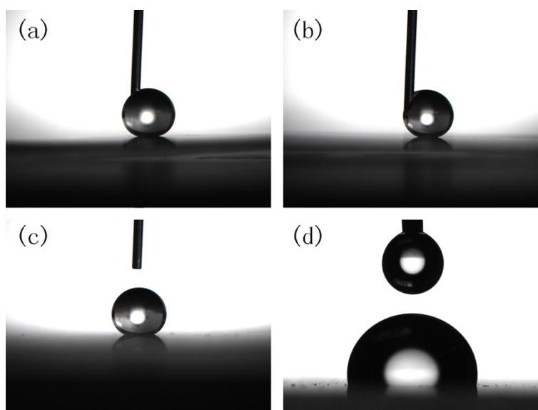
**Figure S3** Water contact angles of  $\text{SiO}_2$  Sol with the sizes of (a) 80 nm, (b) 100 nm, (c) 150 nm and (d) 300 nm
