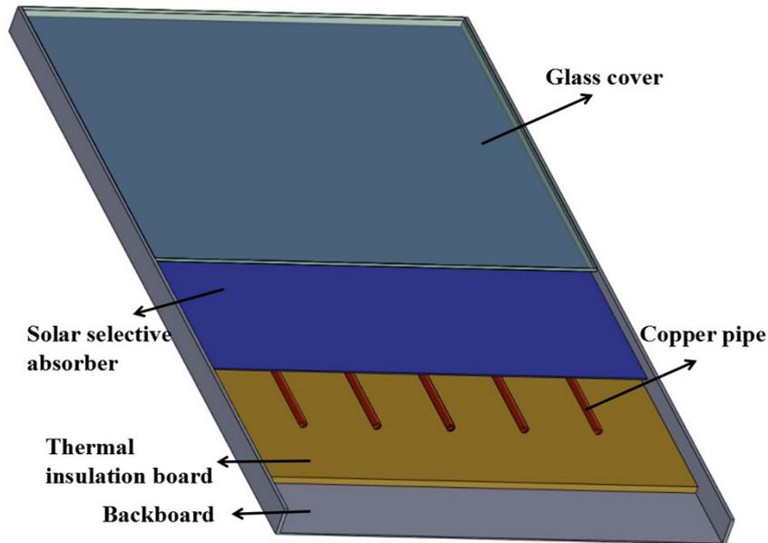
**Figure S1** Structural diagram of flat plate solar collector
