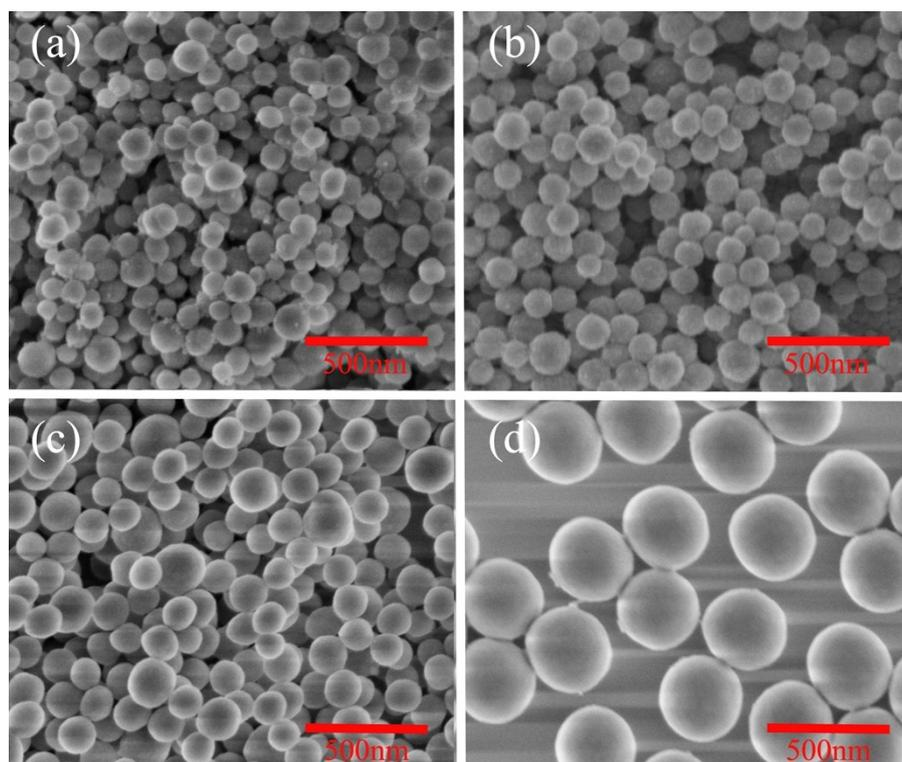
**Figure S2** SEM images of SiO<sub>2</sub> nanoparticles with the sizes of (a) 80 nm, (b) 100 nm, (c) 150 nm and (d) 300 nm
