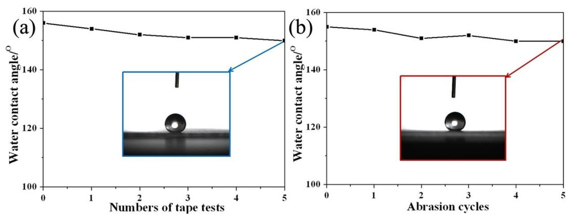
**Figure S6** Water contact angles of the samples with sandwich structure after (a) tape peeling tests and (b) sandpaper abrasion tests
