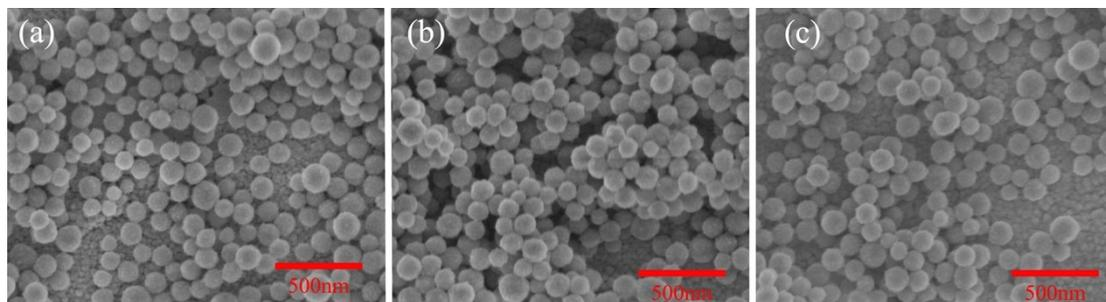
**Figure S4** SEM images of SiO<sub>2</sub> coatings formed by (a) dip-coating, (b) spraying and (c) spin-coating method
