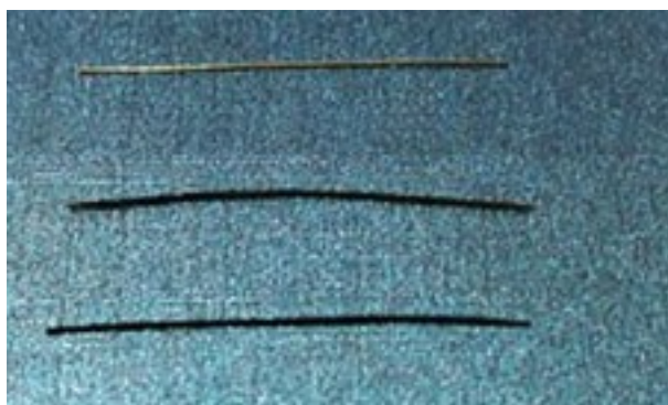
Figure S3. The photos of pure Ti wire, \text{CuCo}_2\text{O}_4/\text{Ti} and \text{CuCo}_2\text{S}_4/\text{Ti} , respectively.
