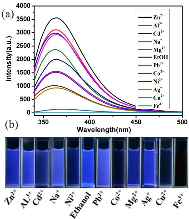
**Fig.S10** (a) Emission spectra of compound **2** in ethanol emulsion containing different metal ions, (b) the luminescence photographs of compound **2** in ethanol emulsion containing different metal ions under UV light.
