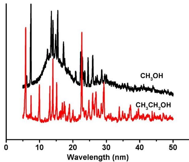
Fig.S1 the PXRD of white powders obtained from the mixed  $\text{CH}_3\text{OH}/\text{H}_2\text{O}$  and  $\text{CH}_3\text{CH}_2\text{OH}/\text{H}_2\text{O}$ , respectively.
