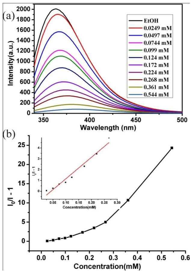
**Fig.S11** (a) fluorescence titration of **2** dispersed in ethanol with the addition of different concentrations of  $\text{Fe}^{3+}$  (excited at 320 nm), (b) the curve of  $(I_0/I - 1)$  vs  $\text{Fe}^{3+}$  concentration in compound **2**. Inset is the linear plot at low concentration.
