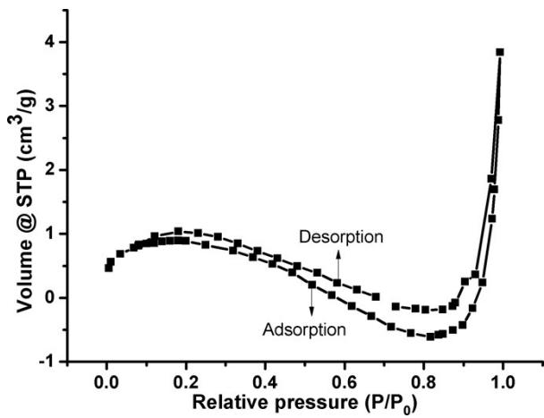
Fig.S12 N<sub>2</sub> adsorption isotherm of compound 2 at 77 K and 1 atm
