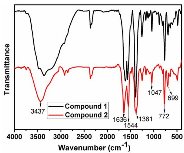
Fig.S8 The IR spectra of compounds **1** and **2**
