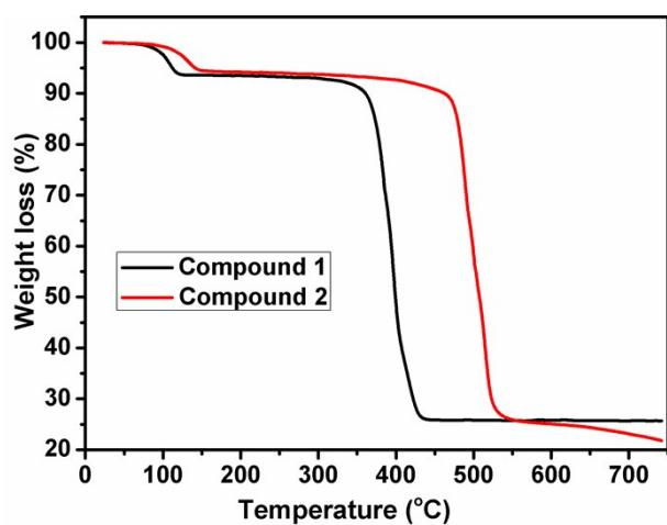
Fig.S9 The TGA curves of compounds **1** and **2**
