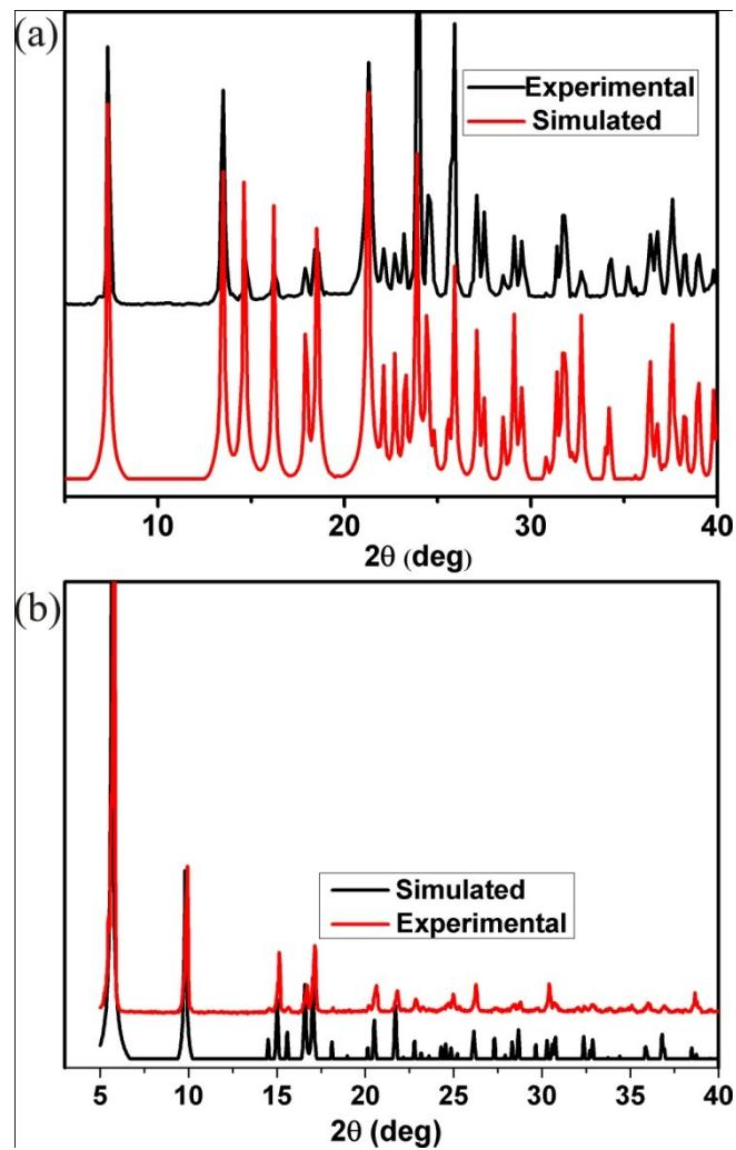
Fig S6. The experimental and simulated X-ray diffraction patterns (a) for compound **1**,
