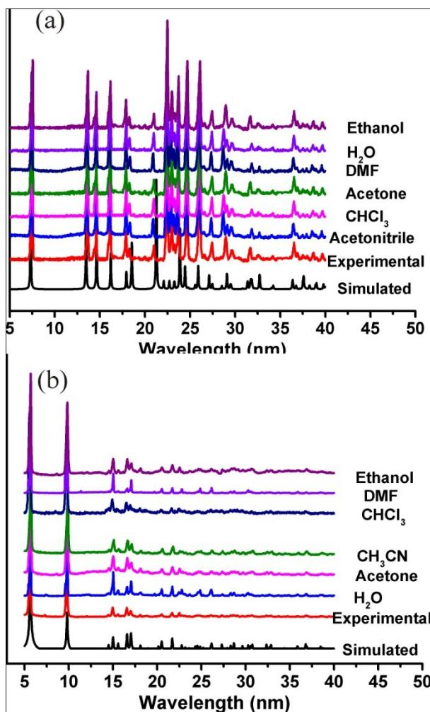
Fig.S7 The Power XRD patterns immersed in different solvents after ultrasonication 30 minutes at room temperature (a) for compound 1, (b) for compound 2
