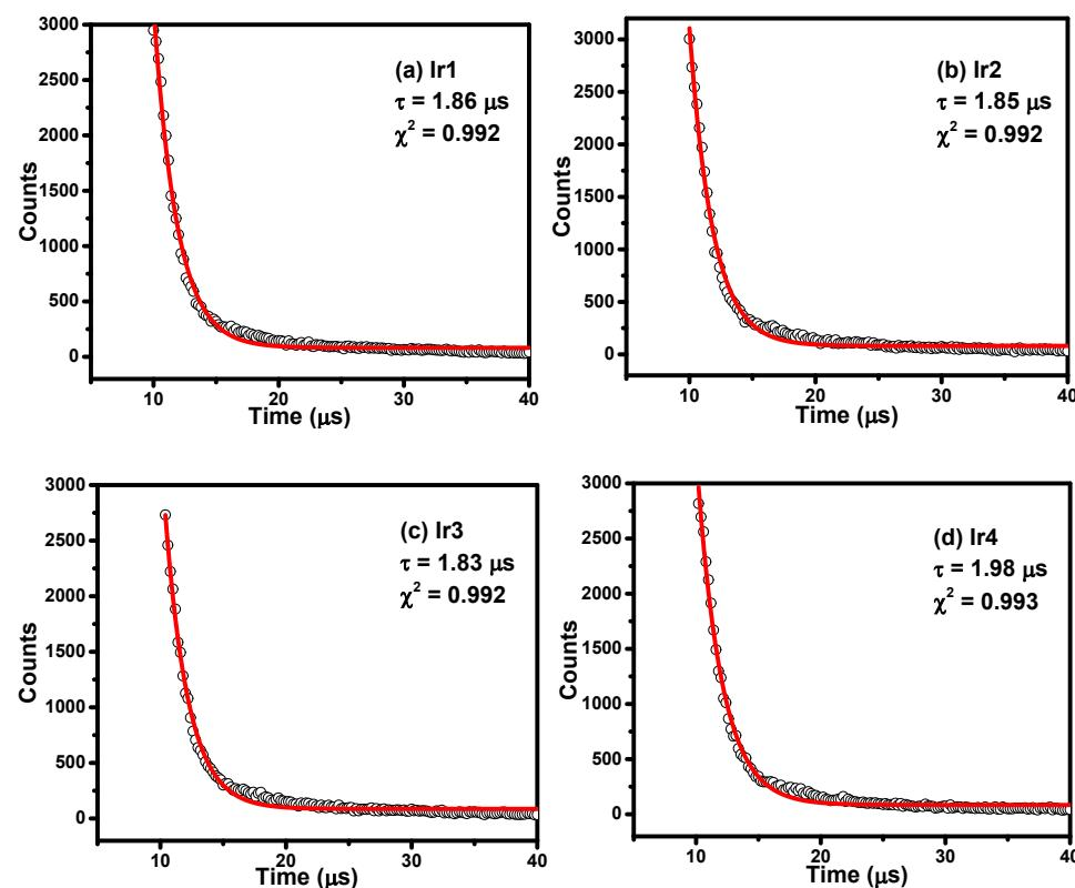
**Fig. S1.** The lifetime curves of (a) **Ir1**, (b) **Ir2**, (c) **Ir3** and (d) **Ir4** in degassed  $\text{CH}_2\text{Cl}_2$  solution at a concentration of  $5 \times 10^{-5} \text{ mol}\cdot\text{L}^{-1}$  at room temperature.
