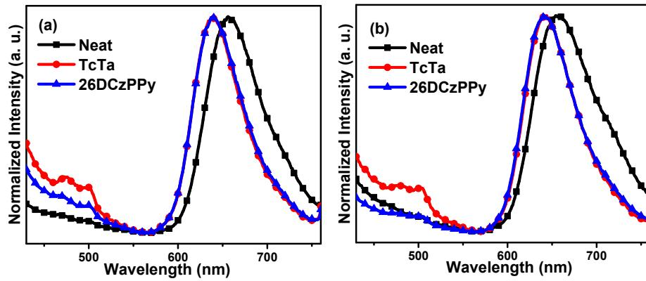
**Fig. S3.** PL spectra in neat and doped films of (a) **Ir3** and (b) **Ir4**.
