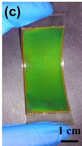
Fig. S4. Bendable green photonic gel film
