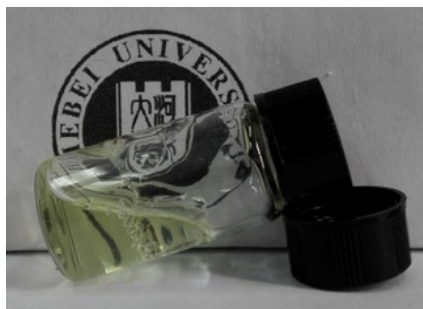
Fig. S2 Hydrogel prepared P(DMA 199 - stat -FPA 4 ) with DTPDH cross-linking.
