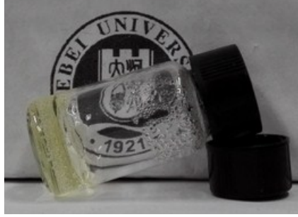
Fig.S3 Hydrogel prepared P(DMA 199 - stat -FPA 4 ) with PEO 90 dihydrazide cross-linking.
