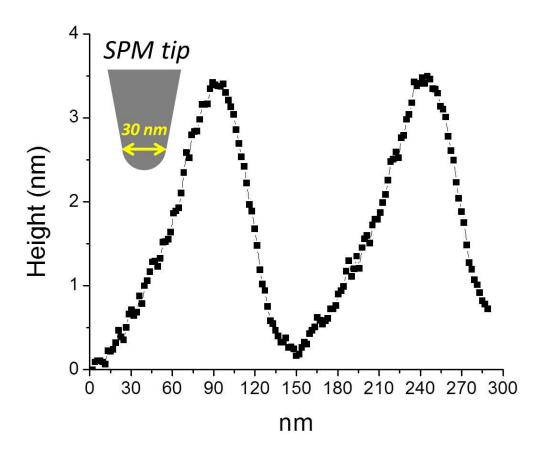
**Figure 4.** The size relation between the apex of the SPM probe and the typical roughness of the CCTO sample (the profile of terrace ledge 2 domain topography is presented).
