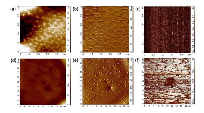
**Figure 3**. A comparison of the topographies (a, d), DFL responses (b, e) and corresponding current distributions (c, f) characteristic of the bump (upper part) and terrace-ledge (bottom part) domain structures (the notation is taken from Ref. 1).
