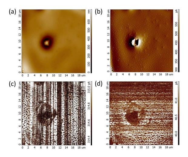
**Figure 6.** Topography (a), DFL response (b) and corresponding top-to-down (c) and left-to-right (d) SR scans. The scan was done at 0.3 Hz (512 x 512 pixels) and dc bias voltage of 1 V.
