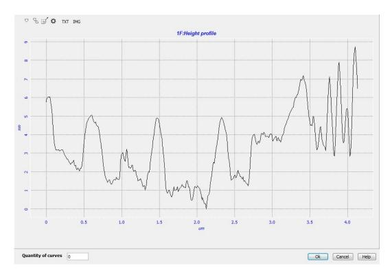
**Figure 1.** Surface topography of mechanically-polished CCTO sample and typical cross-section indicating the RMS roughness of around 5 nm.
