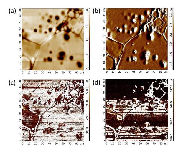
**Figure 2.** Topography (a), DFL response (b) and corresponding SR signal decay due to the degradation of the Pt/Ir coating: new tip (c), the same tip after 3 hours cycling at 0.1 Hz (512 x 512 pixels) (d).
