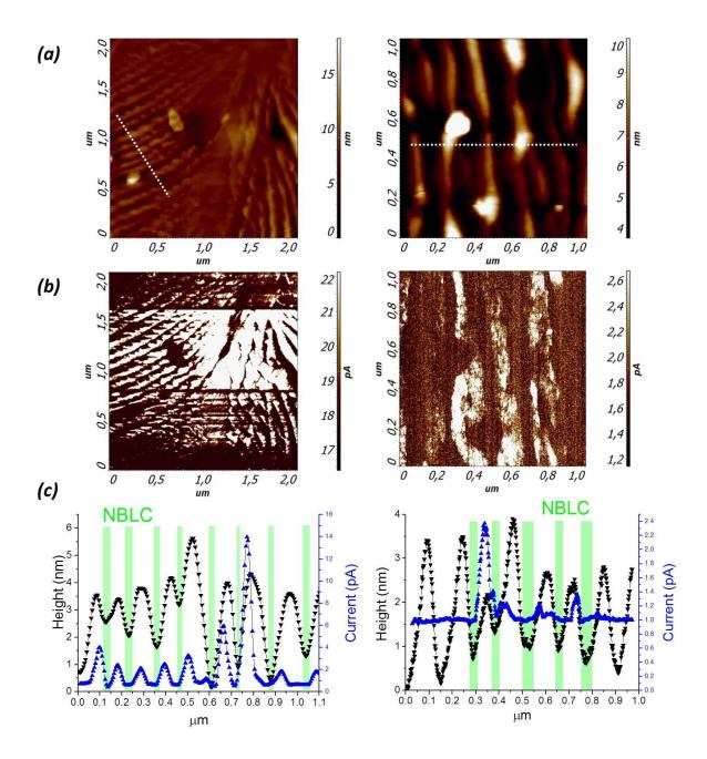
**Figure 5.** Topography (a), corresponding current distribution (b) and their profiles (c) obtained for the terrace ledge 1 (left) and terrace ledge 2 (right) domain areas.
