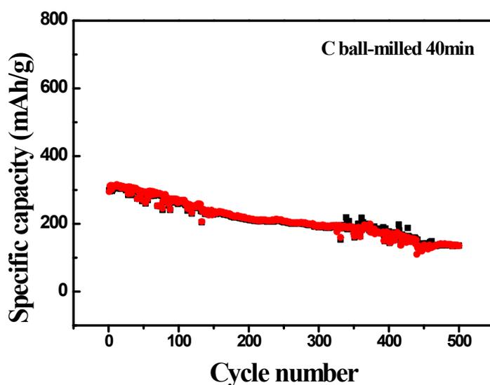
Fig.S3. Cycle performance of C ball-milled 40 min at a current density of  $0.1 \text{ A g}^{-1}$
