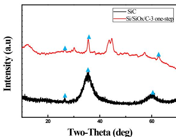
Fig. S2. XRD patterns of pure SiC and Si/SiO<sub>x</sub>/C-3 composite fabricated by one-step ball-milling
