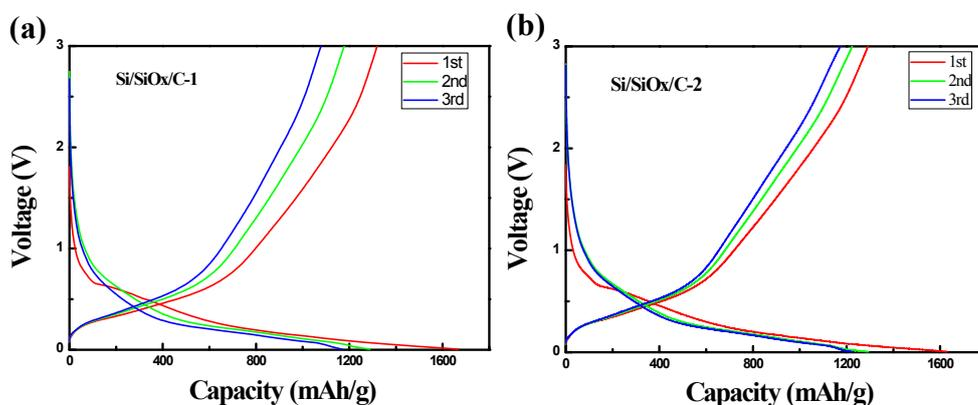
Fig.S4. Charge and discharge voltage profiles of Si/SiO<sub>x</sub>/C-1 and Si/SiO<sub>x</sub>/C-2 at a current density of  $0.1 \text{ A g}^{-1}$
