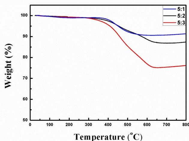
Fig. S1. TGA curve of Si/SiO<sub>x</sub>/C at different weight ratios of Si/SiO<sub>x</sub> to graphite
