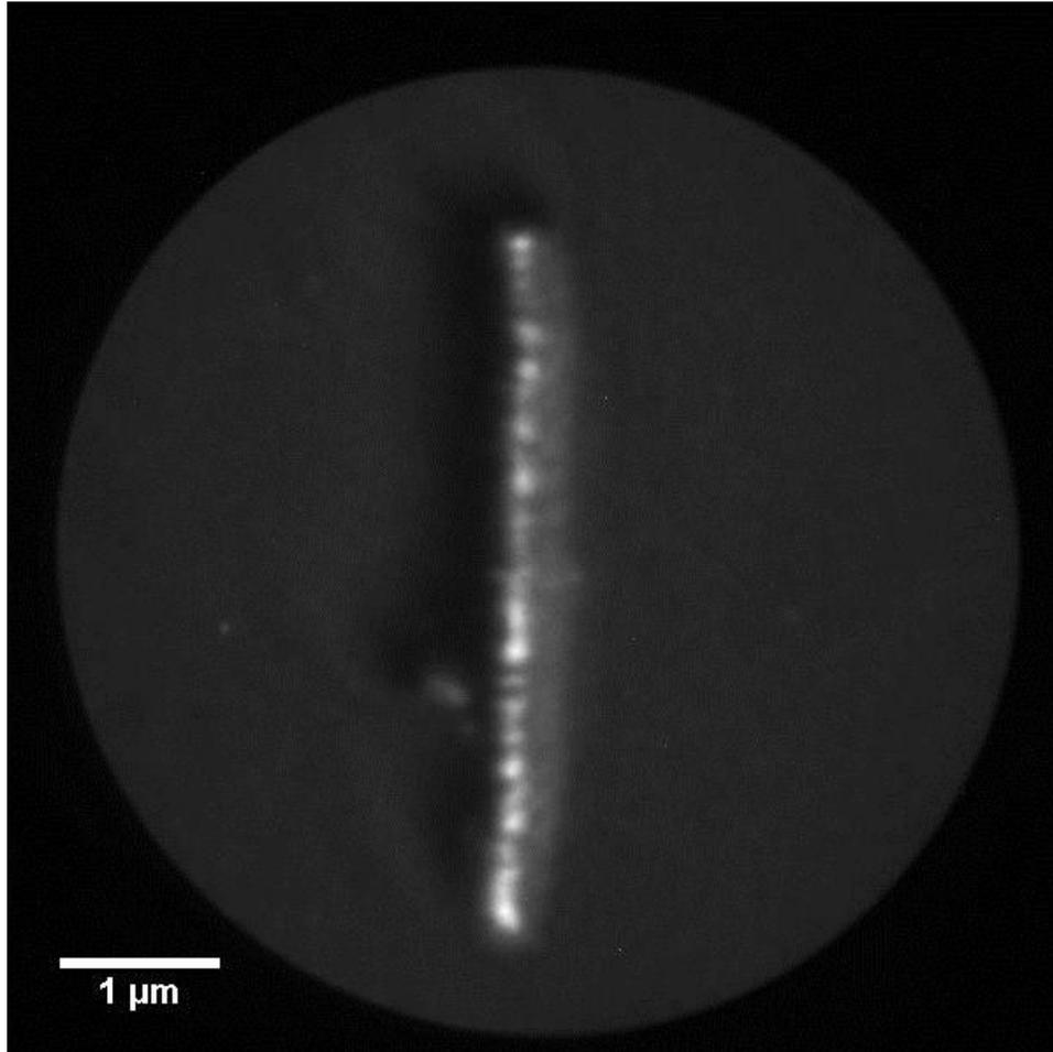
**Figure S4.** Ultraviolet photoemission electron micrograph (UV-PEEM) of an isolated NiCo / Cu wire of 200 nm diameter and with 200 nm segment length.
