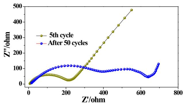
S11 Nyquist plots of the rGO/Si P after 5 cycles and 100 cycles from 100 kHz to 0.01 Hz in the fully charged state.
