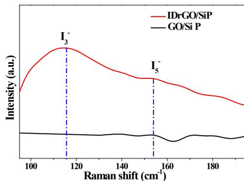
**S2** Two new peaks located at  $116\text{ cm}^{-1}$  and  $154\text{ cm}^{-1}$ , which are absent for both pristine and restored graphene.
