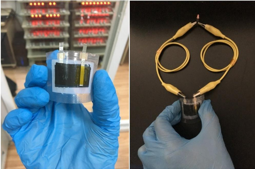
**S7 I-rGO/Si P as a flexible battery was demonstrated by a home-made pouch cell and the flexible device light a red LED.**
