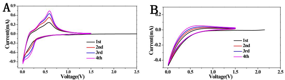
**S8 CV curves of self-supporting Si and I-rGO P in the initial four cycles at scan rate of  $0.1\text{mVs}^{-1}$  in the potential range of 0 to 1.5V (vs.  $\text{Li/Li}^+$ )**
