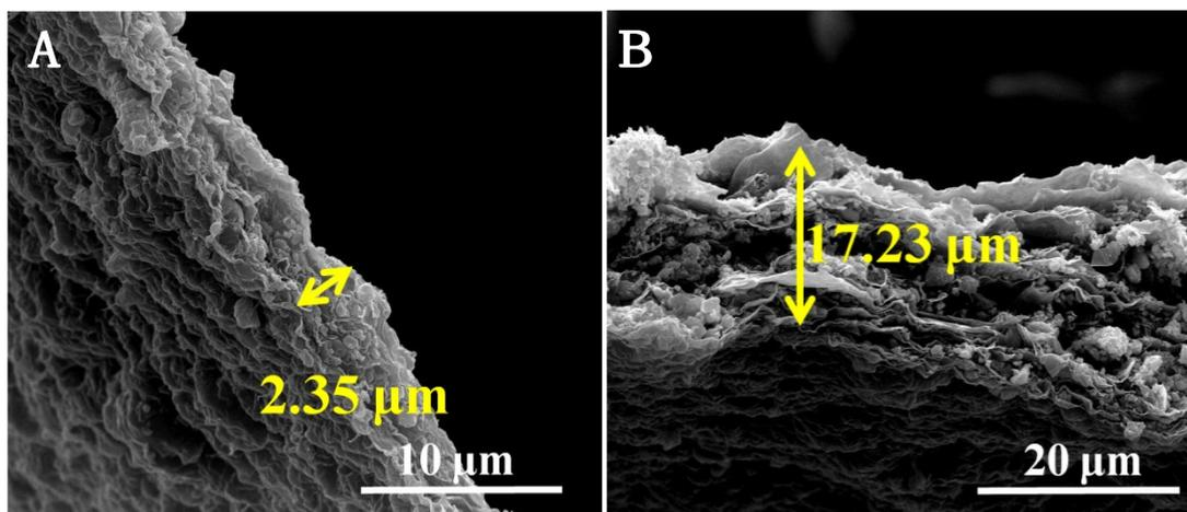
**S4** The cross-sectional SEM images of I doped rGO/Si composite paper by (A) 2ml and (B) 10 ml precursor solution.
