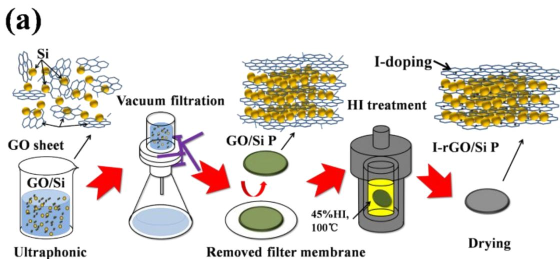
S1 Schematic synthesis of in-situ iodine doped rGO/Si composite paper (I-rGO/Si P).
