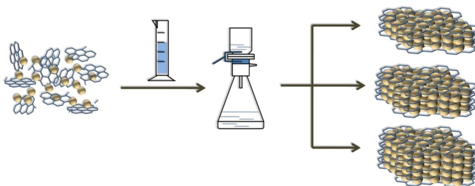
**S3** Direct the controlling of thickness of IDrGO/Si P by the different dosage of precursor solution
