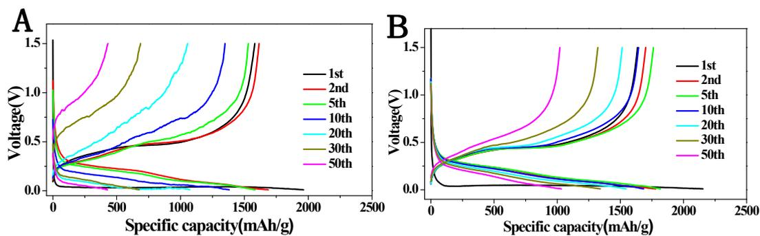
S10 The galvanostatic charge/discharge profiles of rGO/SiP and I-rGO/SiP in the initial 50 cycles
