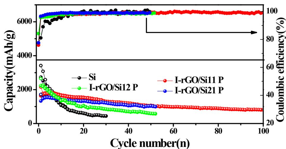
S9 (A) Cycling performance of I-rGO/Si P with different compositions, and the pristine Si for comparison. (B) Cycling performance and coulombic efficiency of the self-supporting I-rGO/Si P with different compositions and the pristine Si at current densities of  $100 \text{ mA} \cdot \text{g}^{-1}$
