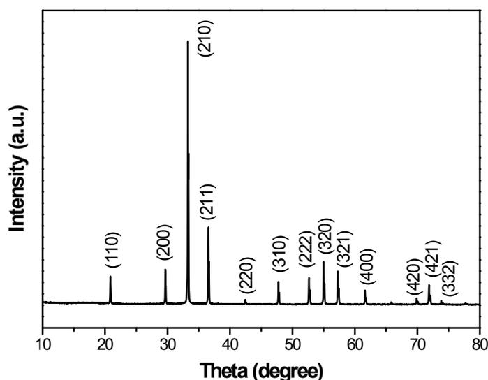
Figure S1. The XRD pattern of  $\text{Ag}_3\text{PO}_4$  nanoparticles. All of the diffraction peaks can be indexed to the cubic structure of  $\text{Ag}_3\text{PO}_4$  (JCPDS card No.06-0505).
