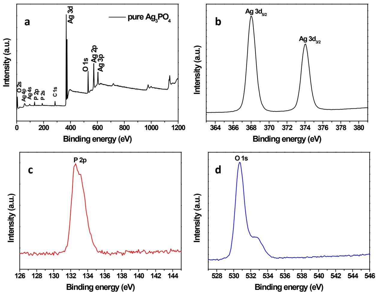
Figure S2. XPS spectra of  $\text{Ag}_3\text{PO}_4$  sample. (a) survey XPS spectrum, (b) Ag 3d, (c) P 2p, (d) O 1s.
