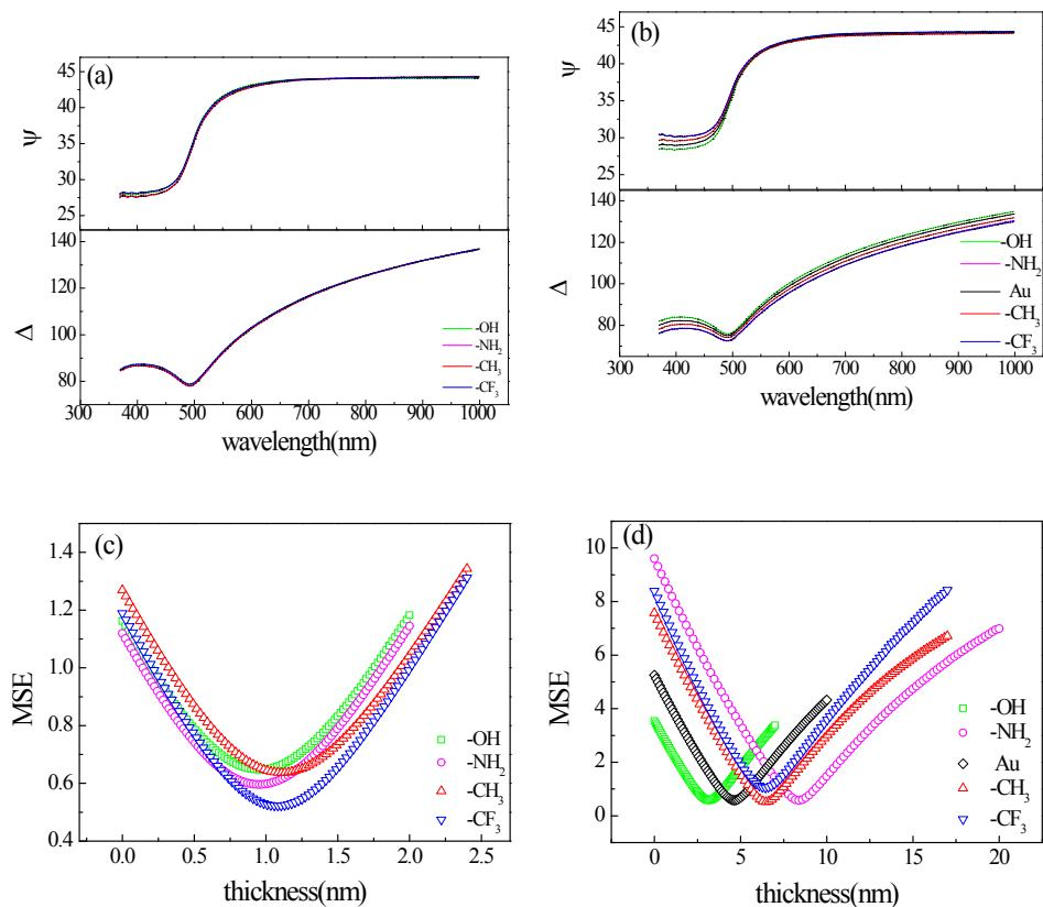
Figure S1. (a) and (b): The plot of  $\Psi$  and  $\Delta$  against  $\lambda$  for Mfp-1 before and after absorbing on the SAMs. The data are fitted by the dash lines. (c) and (d) The plot of mean-square-error against  $h$  for the corresponding samples in (a) and (b).
