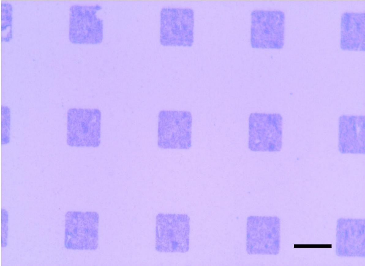
Figure S1: Additional optical micrograph of MoS<sub>2</sub> on patterned graphene. Scale bar corresponds to 20  $\mu\text{m}$ .
