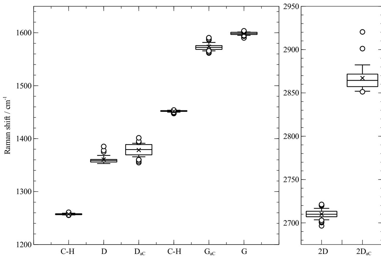
Figure S3: Statistical dispersion of Raman peak positions based on fitting of multiple ( $N = 24$ ) MoS<sub>2</sub>-on-graphene Raman spectra. Cross indicates mean position, box indicates the upper and lower quartiles, and the whiskers denote the standard deviation. Circles indicate outliers.
