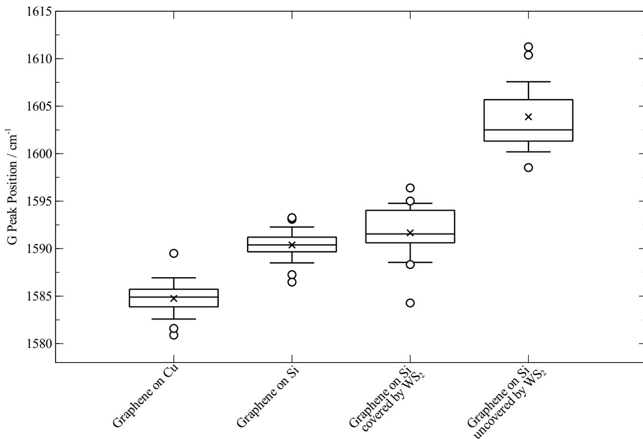
Figure S5: Box plot of Raman G peak position at different stages of WS<sub>2</sub>-on-graphene growth process. Upshift indicates doping level, which is significant for graphene after WS<sub>2</sub> CVD, but not covered by WS<sub>2</sub>.  $N = 12$
