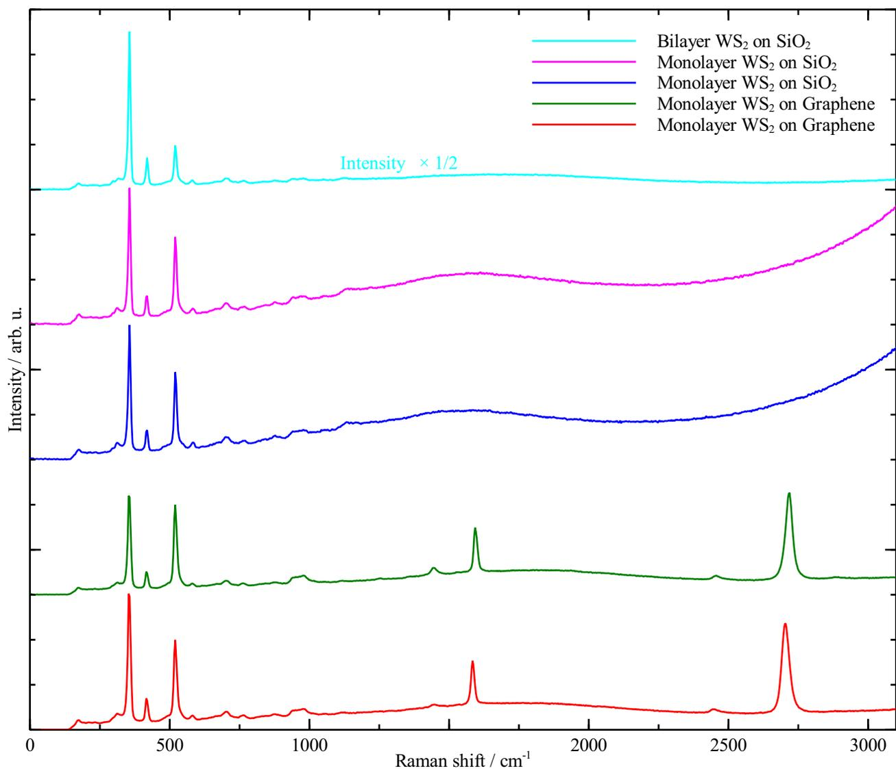
Figure S6: Onset of fluorescence tail near  $3000\text{ cm}^{-1}$  offer additional evidence that identification of monolayer  $\text{WS}_2$  is correct.
