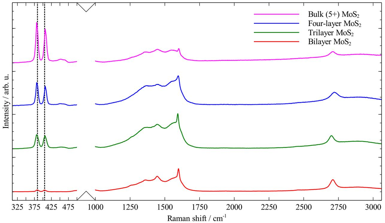
Figure S2: Raman spectrum of MoS<sub>2</sub> on graphene ranging from bilayer to bulk (5+ layers).
