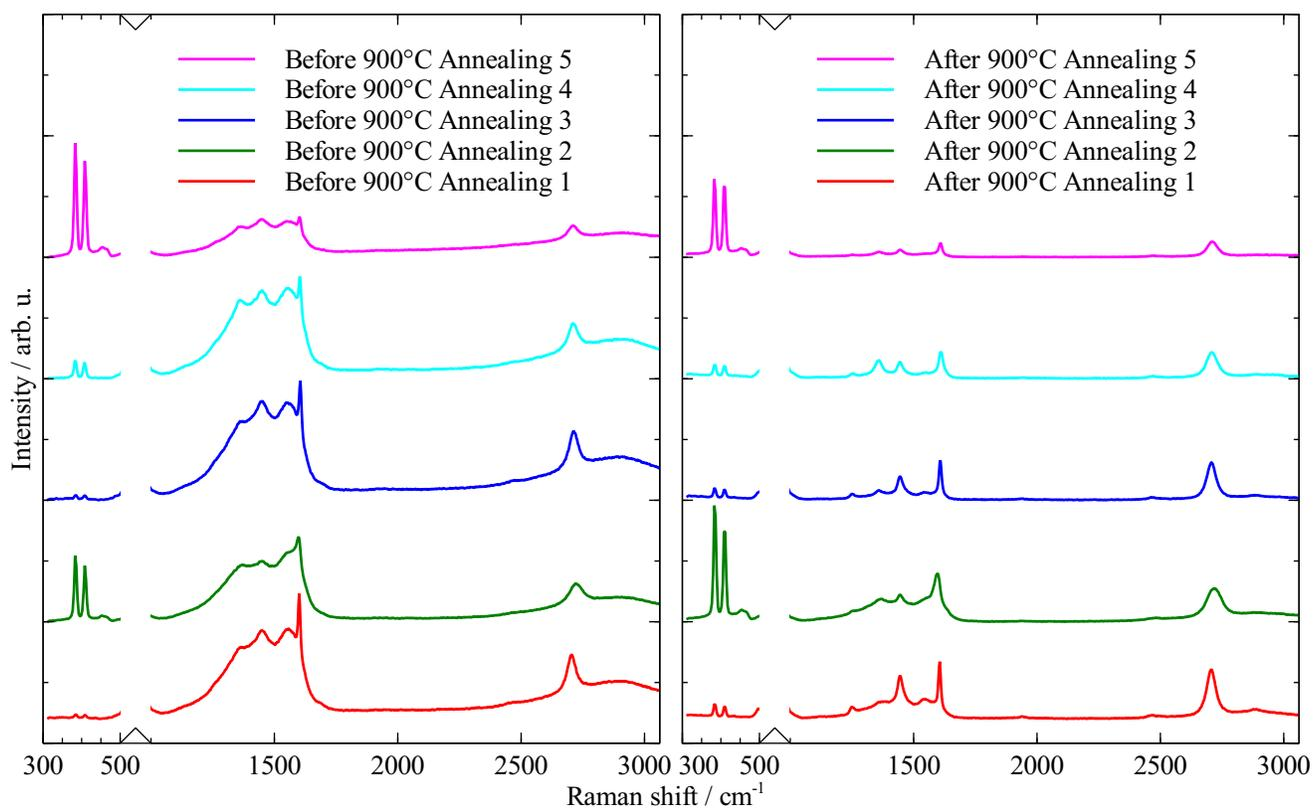
Figure S4: Left panel: Raman spectra of MoS<sub>2</sub> grown on graphene. Right panel: Raman spectra of MoS<sub>2</sub>-on-graphene after annealing in sulfur environment at 900 °C. Spectra in left and right panels were taken at the same positions.
