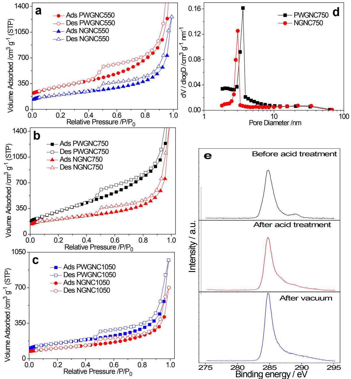
Figure S2. Nitrogen adsorption/desorption isotherms of GNCs before and after removal of doping template: NGNC550 and PWGNC550 (a), NGNC750 and PWGNC750 (b), and NGNC1050 and PWGNC1050 (c). (d) Mesopore distribution (BJH) of NGNC750 and PWGNC750. (e) XPS C1s spectra of GNC-precursor (before acid treatment), NGNCs (after acid treatment) and PWGNCs (after vacuum).
