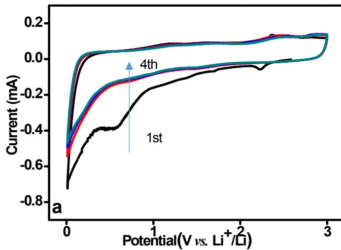
Figure S3. Cyclic voltammetry (CV) profile of PWGNC700 at a scan rate of 0.1mV/s between 0.01-3V versus Li<sup>+</sup>/Li for the 1st-4th charge/discharge cycles.
