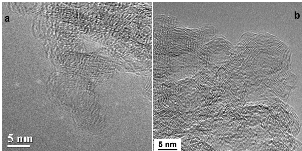
Figure S1. HRTEM image of the PWGNCs prepared at 550 °C (a) and 1050 °C (b)
