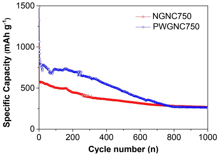
Figure S5. Cycling performance of the NGNC750 and PWGNC750 based electrodes at a current density of  $4 \text{ A g}^{-1}$ .
