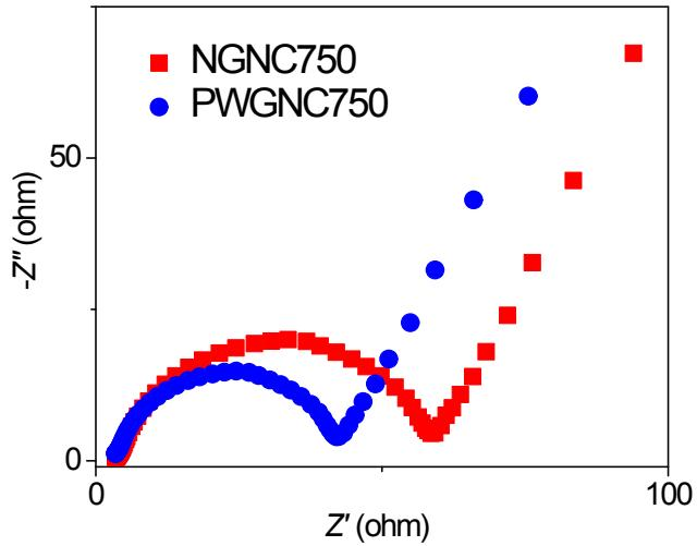
Figure S4. AC impedance plots for NGNC750 and PWGNC750
