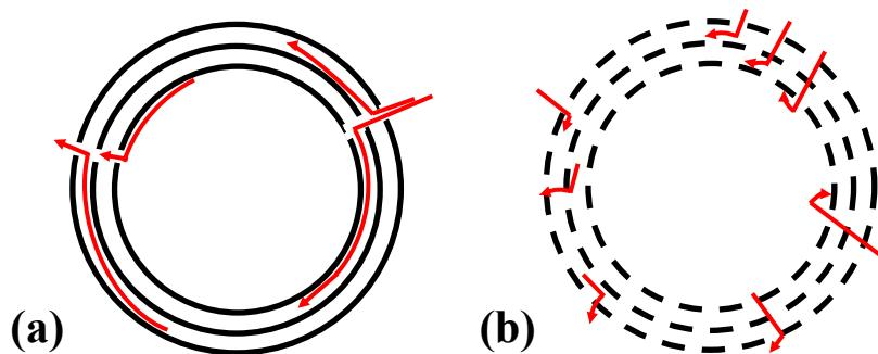
Figure S6. Effect of highly nanoporous graphitic shells of GNCs: shortening diffusion route of electrolyte ions. GNCs without (a) and with (b) removal of doping template.
