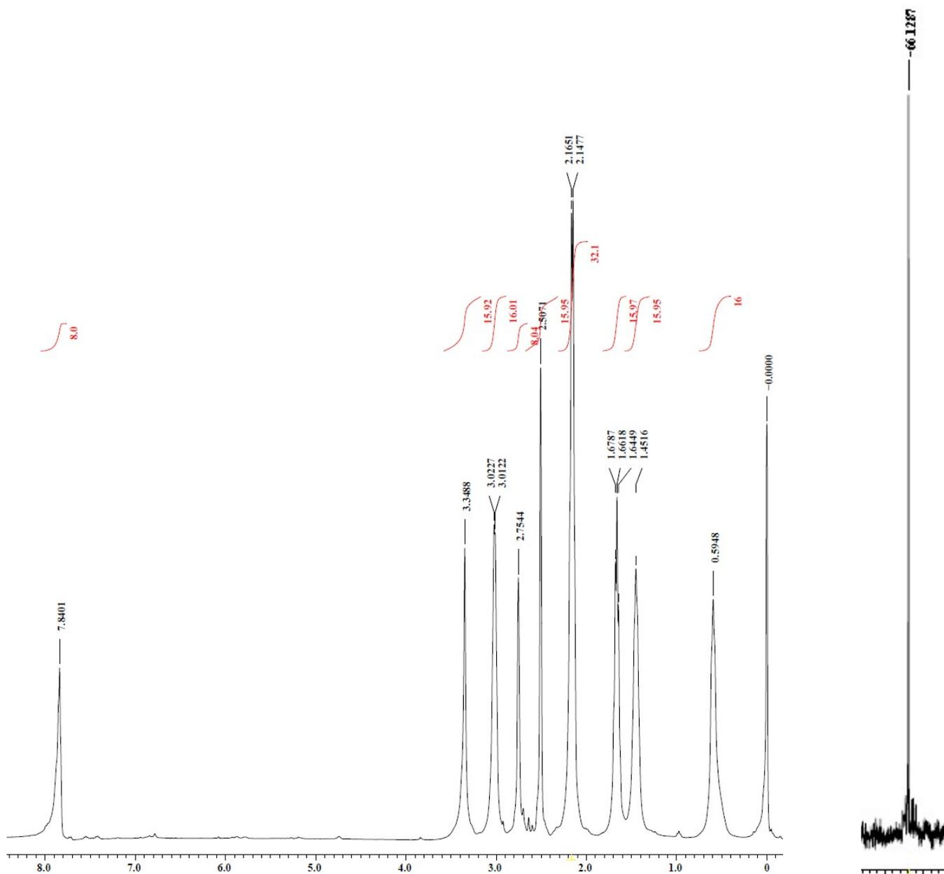
**Figure S1.**  $^1\text{H}$  NMR and  $^{29}\text{Si}$  NMR spectra of  $T_8[N\text{-propyl-hex-5-ynamide}]_8$  (2)
