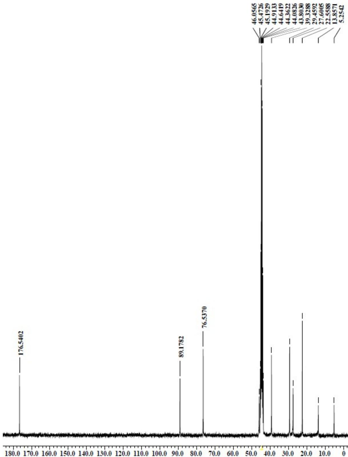
Figure S2.  $^{13}\text{C}$  NMR spectrum of  $\text{T}_8[\text{N-propyl-hex-5-ynamide}]_8$  (2)
