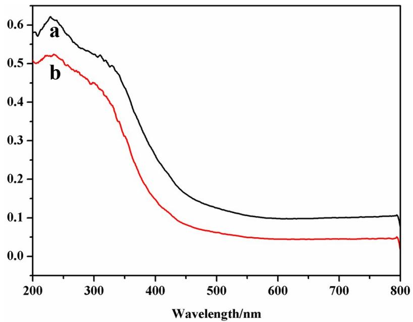
**Fig. S4** The DR-UV-vis spectra of (a)  $C_{16}PW(O_2)_2/PNIPAM$ , and (b)  $C_{16}PW(O_2)_2/PNIPAM$  after the degradation of phenol
