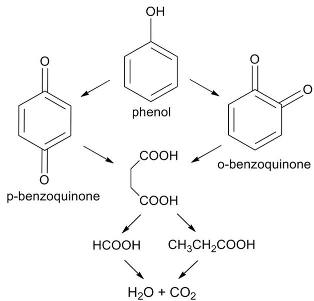
**Scheme S1** The possible degradation of phenol in CWPO process using  $C_{16}PW(O_2)_2/PNIPAM$  as catalyst
