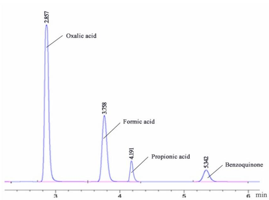
**Fig. S7** The high performance liquid chromatography (HPLC) of intermediate products
