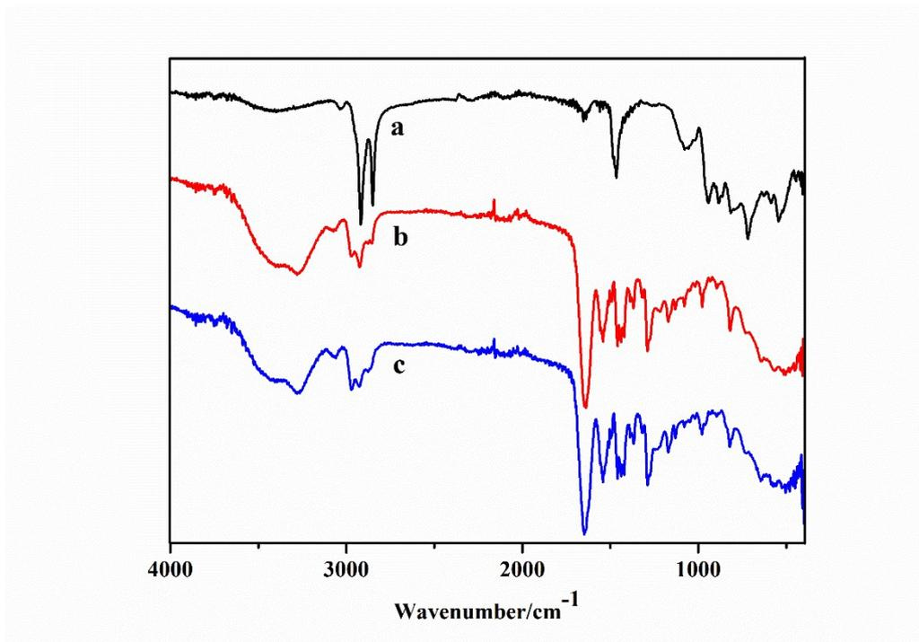
**Fig. S3** The IR spectra of (a)  $C_{16}PW(O_2)_2$ , (b)  $C_{16}PW(O_2)_2/PNIPAM$ , and (c)  $C_{16}PW(O_2)_2/PNIPAM$  after the degradation of phenol.
