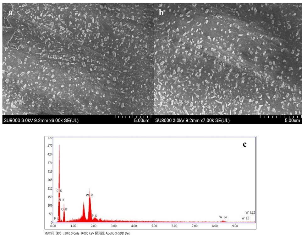
**Fig. S6** The SEM images of (a) fresh  $C_{16}PW(O_2)_2/PNIPAM$ , (b)  $C_{16}PW(O_2)_2/PNIPAM$  after the reaction, and (c) the EDAX spectrum of fresh  $C_{16}PW(O_2)_2/PNIPAM$ .
