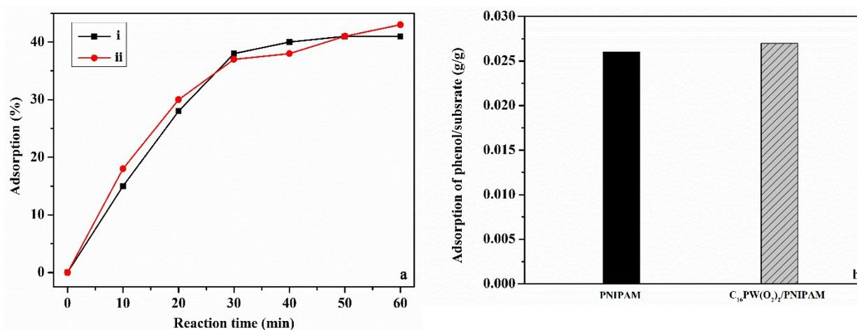
**Fig. S1** (a) The changes of phenol adsorption on PNIPAM (i) and C<sub>16</sub>PW(O<sub>2</sub>)<sub>2</sub>/PNIPAM (ii); (b) The maximum adsorption amount of phenol per gram of PNIPAM in pure polymer and in C<sub>16</sub>PW(O<sub>2</sub>)<sub>2</sub>/PNIPAM. Reaction conditions: PNIPAM (0.0084 g), C<sub>16</sub>PW(O<sub>2</sub>)<sub>2</sub>/PNIPAM (0.01 g), phenol solution (0.72 mM, 5 mL), 25 °C.
