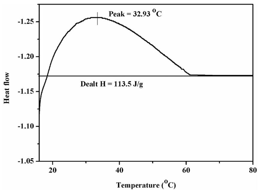
**Fig. S2** The DSC curve of C<sub>16</sub>PW(O<sub>2</sub>)<sub>2</sub>/PNIPAM.
