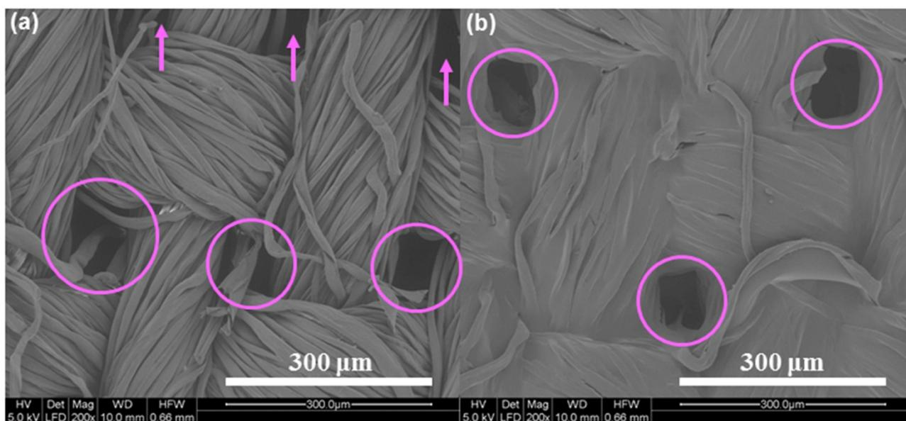
**Supplementary Fig. S1** SEM images of commercial cotton fabric (a) before and (b) after PEDOT:PSS coating treatment. The holes between the warp direction and weft direction of the commercial cotton fabric was marked by pink arrows and pink circles in the Fig. S1 (a) and (b).
