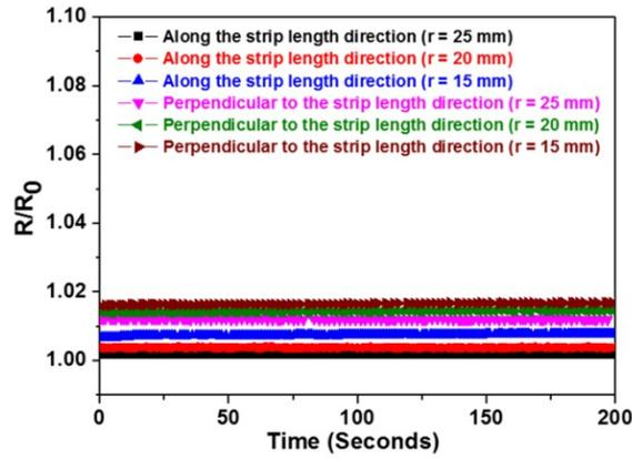
**Supplementary Fig. S11** Effects of bending at different radii and directions on the internal resistance of the fabric-based TE power generator.
