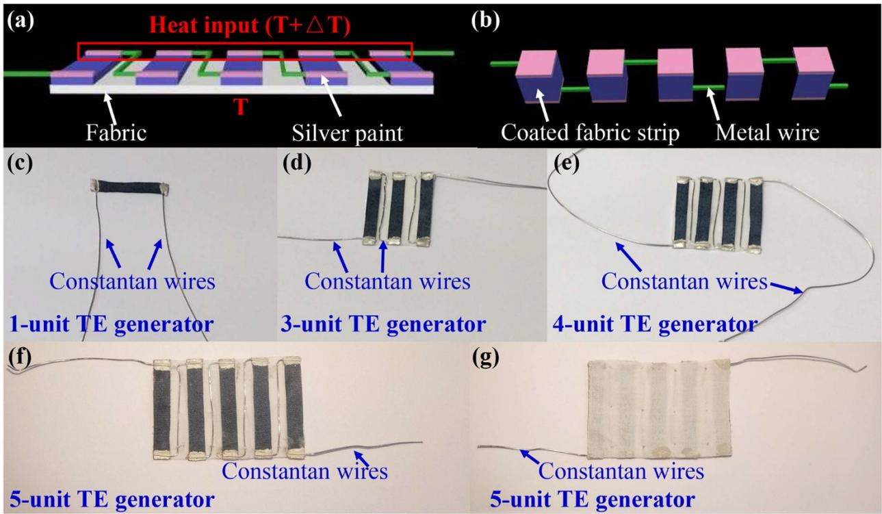
**Supplementary Fig. S6** Schematic illustration of the fabric-based TE generators, (a) I-type connection, and (b)  $\pi$ -type connection. Positive face of the fabric-based TE generators connected with Constantan wires, (c) 1-unit, (d) 3-unit, (e) 4-unit, and (f) 5-unit. Negative face of the fabric-based TE generators connected with Constantan wires, (g) 5-unit.
