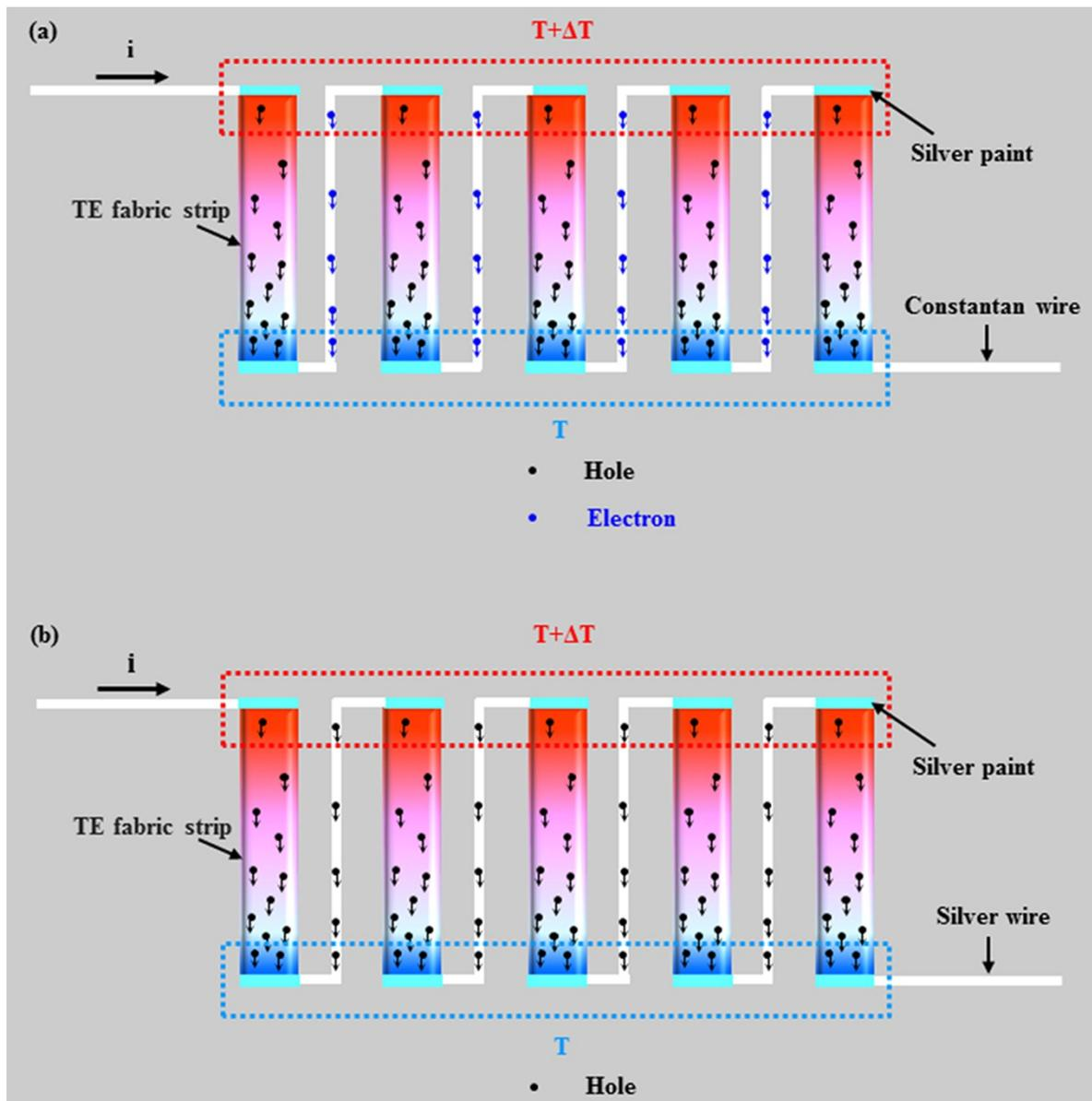
**Supplementary Fig. S8** Schematic illustrations of micromechanism of fabric TE generator connected with (a) Constantan wires and (b) silver wires.
