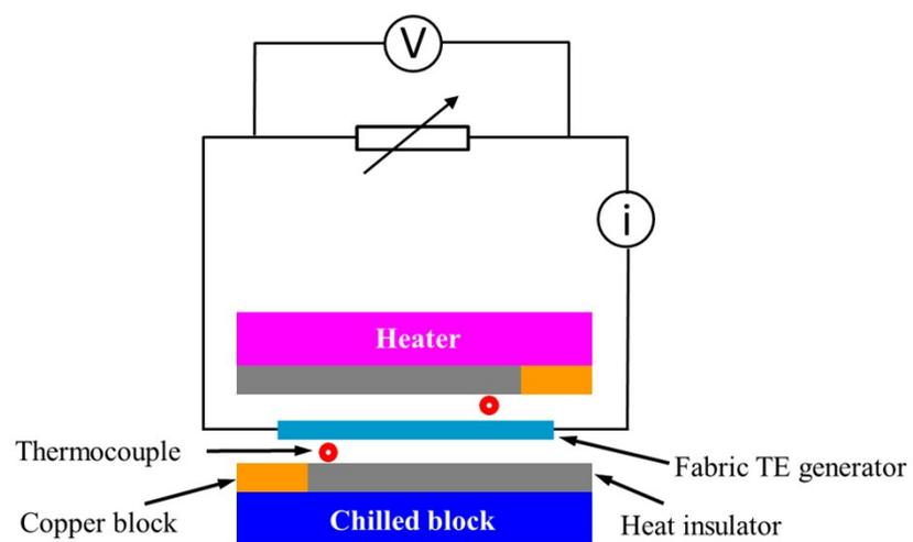
**Supplementary Fig. S7** Schematic illustration of the measurement setup for evaluate the performance of the fabricated fabric-based TE generator
