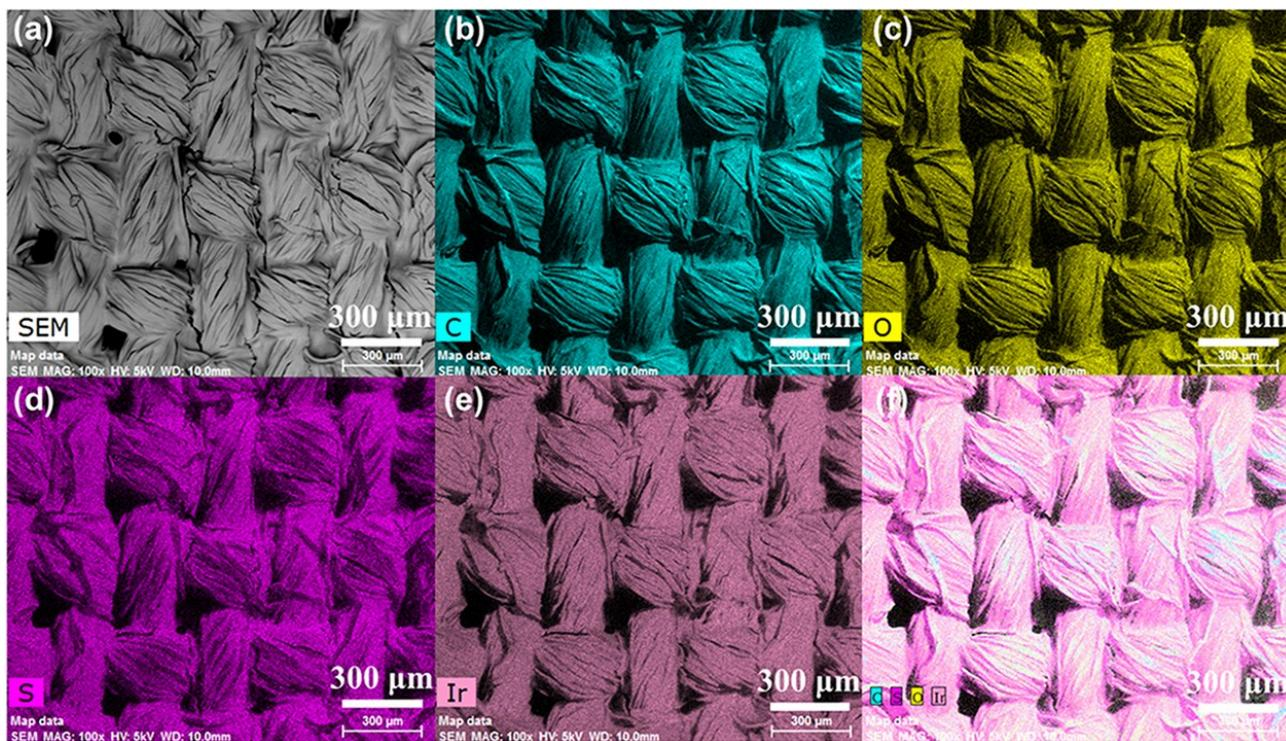
**Supplementary Fig. S3** (a) SEM image and (b) - (f) SEM-EDS mapping images of the PEDOT:PSS coated cotton fabric.
