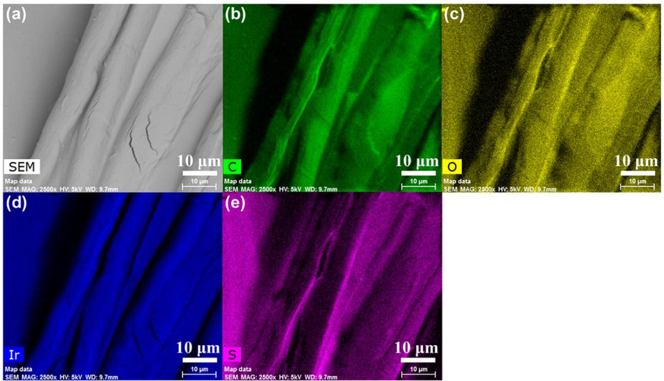
**Supplementary Fig. S4** (a) SEM image and (b) - (e) SEM-EDS mapping images of the PEDOT:PSS coated cotton fibers.
