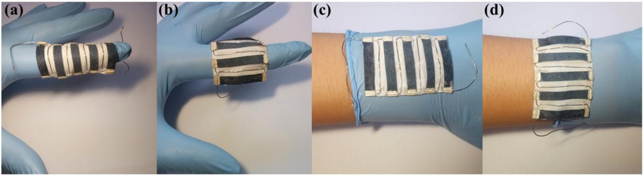
**Supplementary Fig. S9** Photos of fabric-based TE generators connected with Constantan wires on the fingers (a) & (b), and (c) & (d) wrists.
