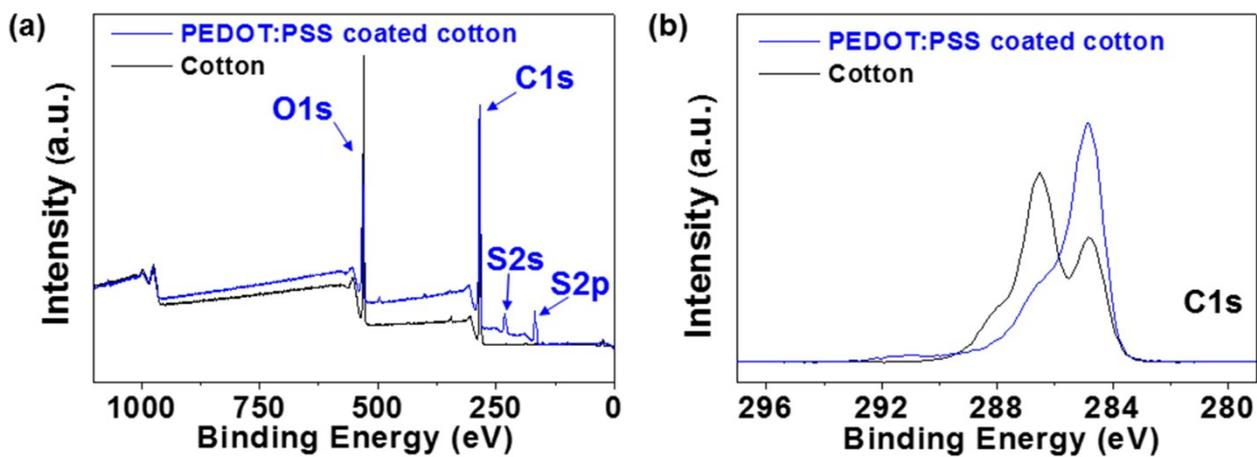
**Supplementary Fig. S5** (a) XPS survey spectra and (b) high resolution C1s spectra of cotton fabric before and after PEDOT:PSS coating treatment.
