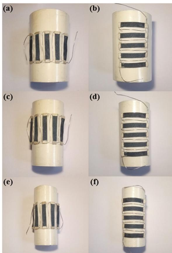
**Supplementary Fig. S10** Photos of the prepared device attached on the surface of the cylinders with different radius (a) & (b) 25 mm, (c) & (d) 20 mm, and (e) & (f) 15 mm.
