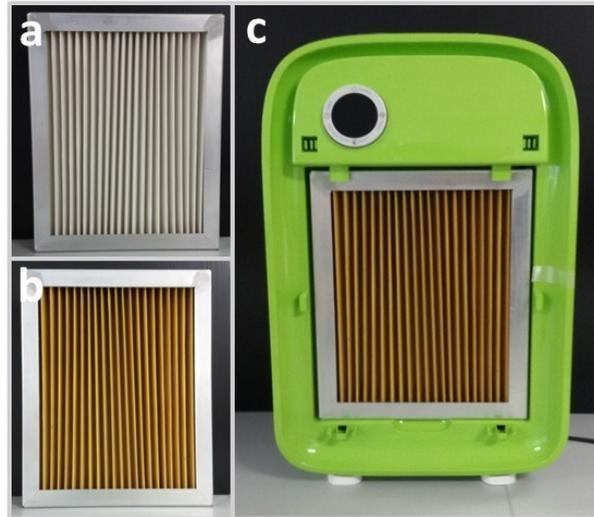
**Figure S7.** Pictures of nanofilter after pleating and framed at (a) back side, (b) front side and (c) nanofilter assemble inside the commercial air filtration machine.
