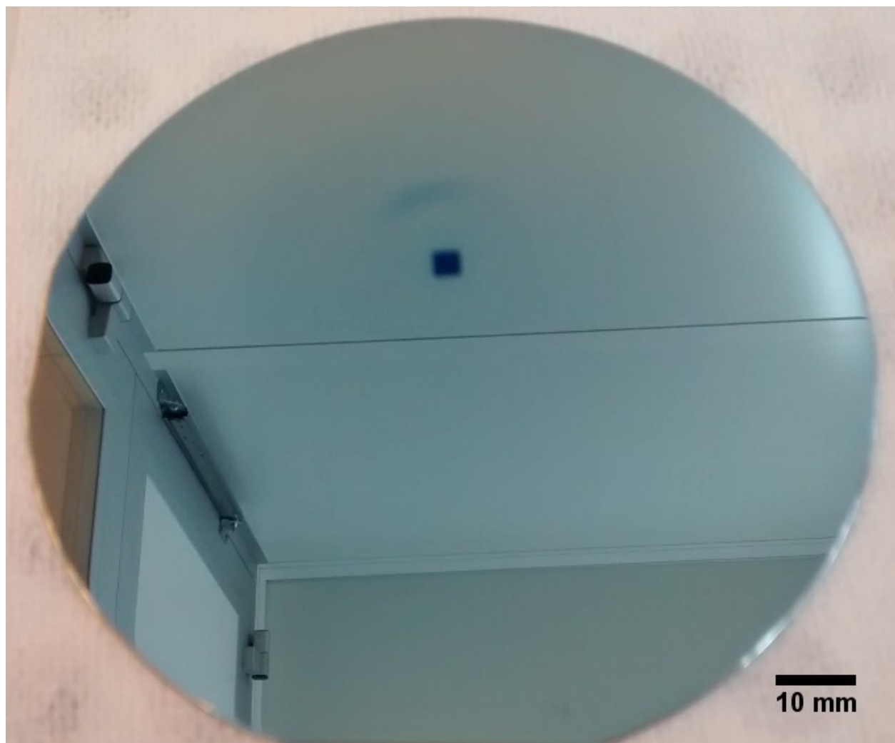
Figure 4: Photo of a wafer after a deposition with humid oxygen at 130°C indicating the homogeneous deposition of the complete wafer surface. The dark square above the center of the wafer and the veil above it occur due to the sputtering prior to XPS measurement
