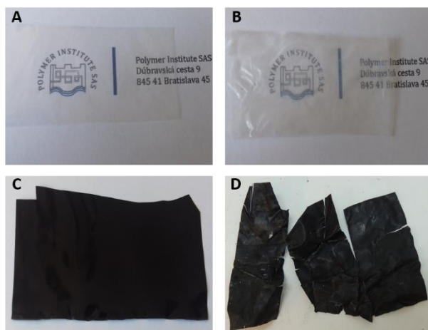
Figure S1: Photos of PLA/PHB (A,B) and PLA/PHB/CB (C,D) foils after preparation (A,C) and after 1 year of mineralization at 20 °C (B,D).
