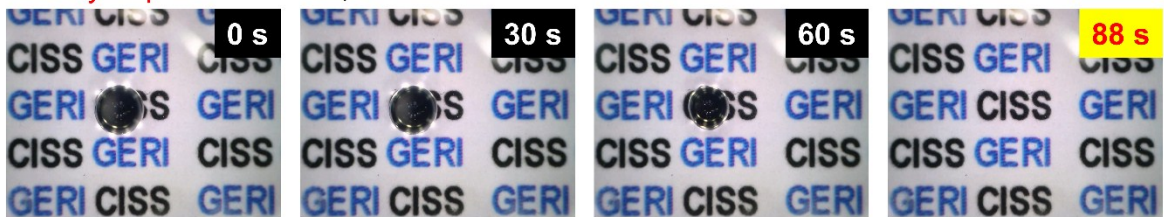
Fig. S6 Evaporation process of water droplets on the surfaces of the Ni mesh-based transparent heaters with different wetting properties at 95 °C.
