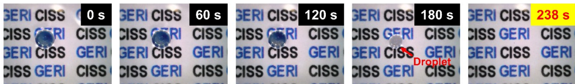
Fig. S5 Evaporation process of water droplets on the surfaces of the Ni mesh-based transparent heaters with different wetting properties at 65 °C.
