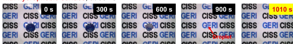
Fig. S3. Evaporation process of water droplets on the surfaces of the Ni mesh-based transparent heaters with different wetting properties at 30 °C.
