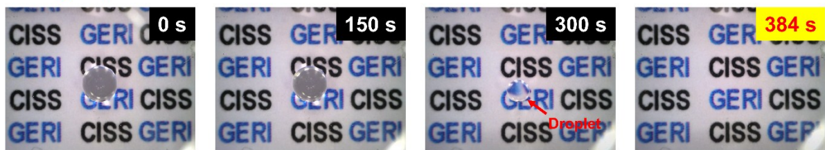
Fig. S4 Evaporation process of water droplets on the surfaces of the Ni mesh-based transparent heaters with different wetting properties at 45 °C.
