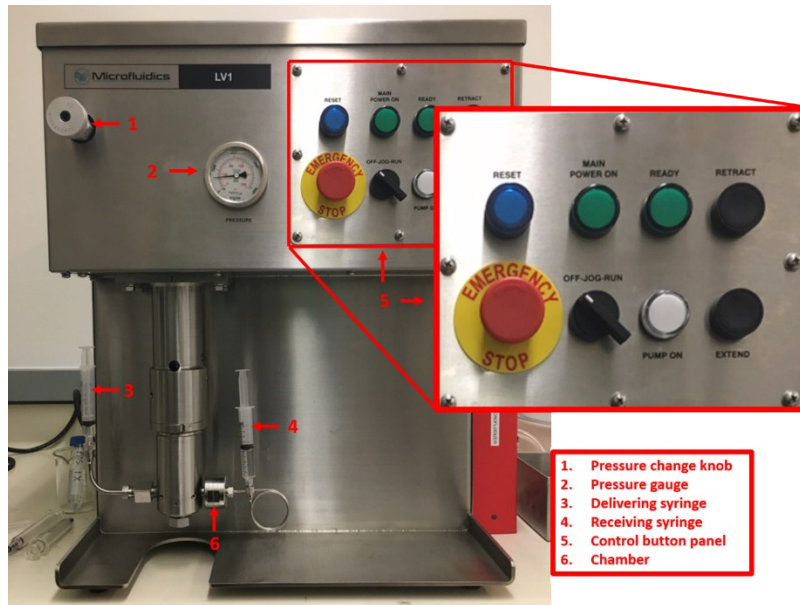
FIGURE S1. Specific components and operating parameters of the high-pressure homogenizer.
