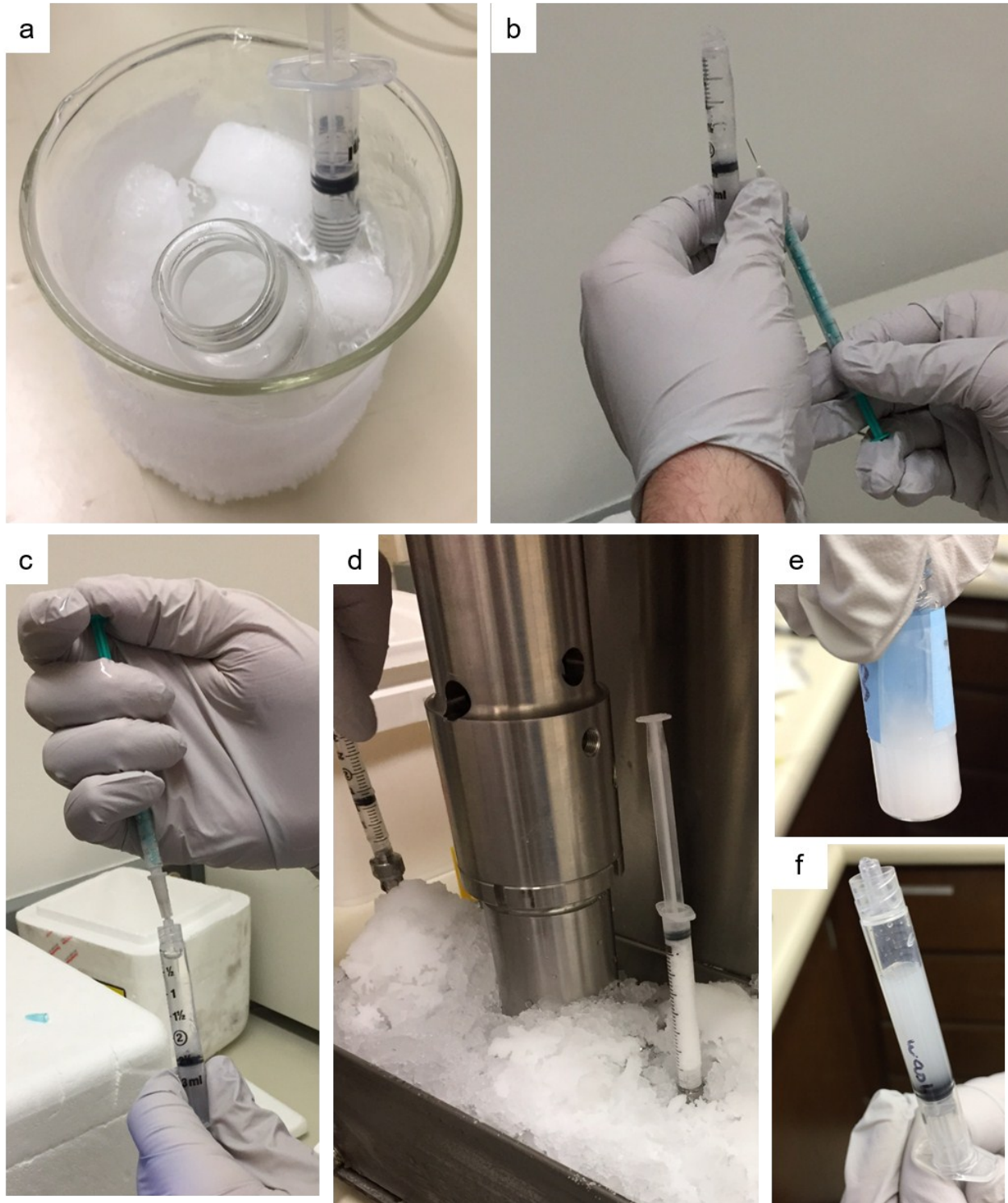
FIGURE S3. Formulation of OFP nanodroplets. a) OFP gas condensed by cooling at -70\text{ }^{\circ}\text{C} using an ethanol-dry ice bath alongside a syringe containing clear lipid film dispersed in excipient
