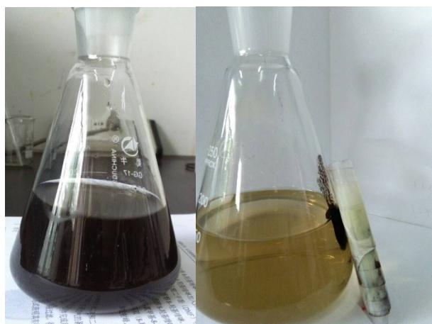
Figure S4. Recycling of Fe-C 500 by using a magnet after 4 cycles.
