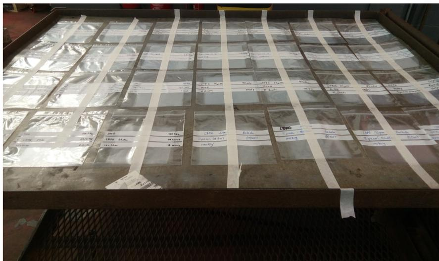
**Figure S1** ETFE films (and other materials for other studies) loaded onto the trolley that moves through the 4.5 MeV Dynamatron Continuous DC electron beam (Synergy Health, South Marston, UK): the length of the beam (40 inch) is the width of the trolley, while the  $e^-$ -beam is  $\frac{3}{4}$  inch in thickness.
