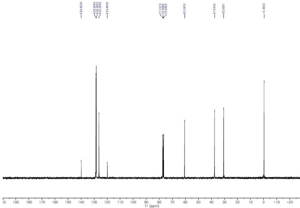
**Figure S69.** <sup>13</sup>C NMR spectrum of 4-phenyl-2-((trimethylsilyl)oxy)butanenitrile in CDCl<sub>3</sub> (Table 4, entry 8)
