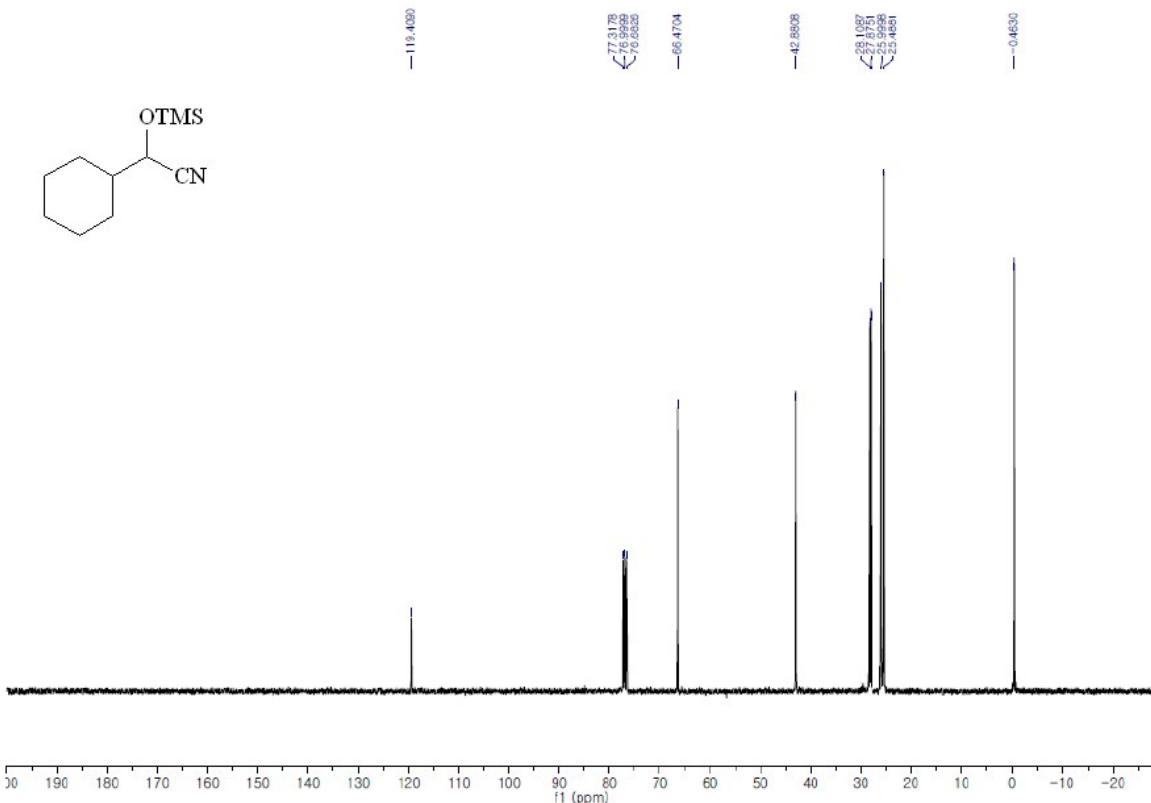
**Figure S73.**  $^{13}\text{C}$  NMR spectrum of 2-cyclohexyl-2-((trimethylsilyl)oxy)acetonitrile in  $\text{CDCl}_3$
