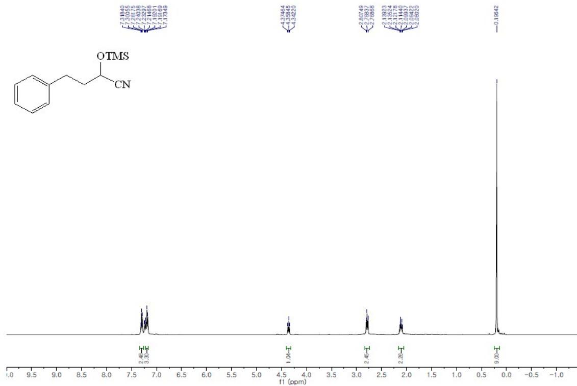
**Figure S68.** <sup>1</sup>H NMR spectrum of 4-phenyl-2-((trimethylsilyl)oxy)butanenitrile in CDCl<sub>3</sub> (Table 4, entry 8)
