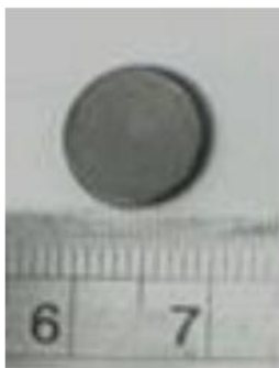
Fig. S2 Sample picture of rGO pellet prepared by pressed equipment
