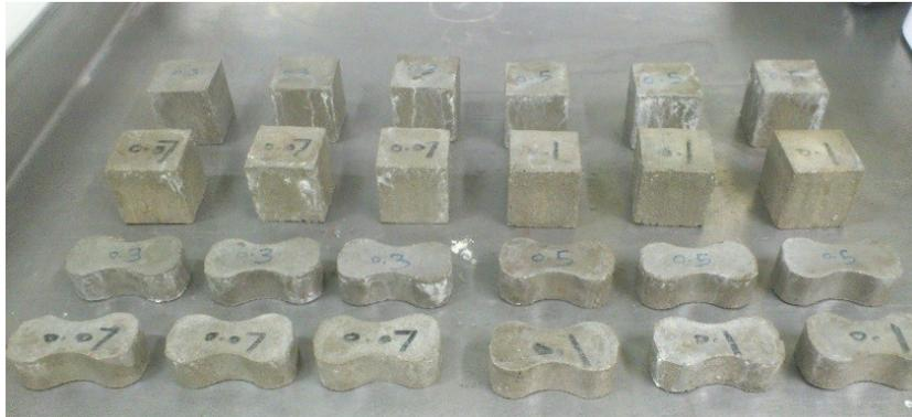
Fig. S2. GO-cement mortar composite samples.
