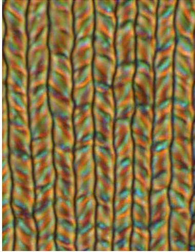
**Figure SI-6:** Photomicrograph (x200) of a region of **A6** showing the rope-like texture.
