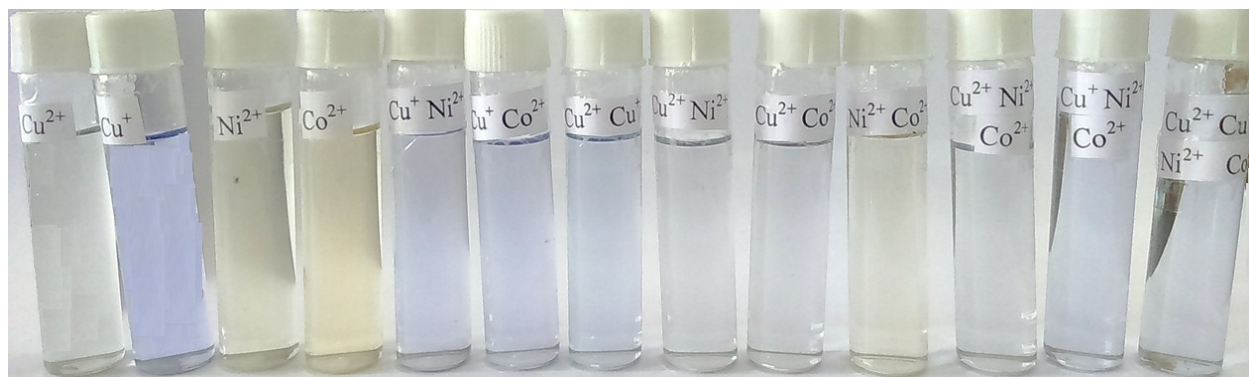
Fig. S18 Color changes observed to Chemosensor H-3 and metal ions ( 1 \times 10^{-4} M) in methanol
