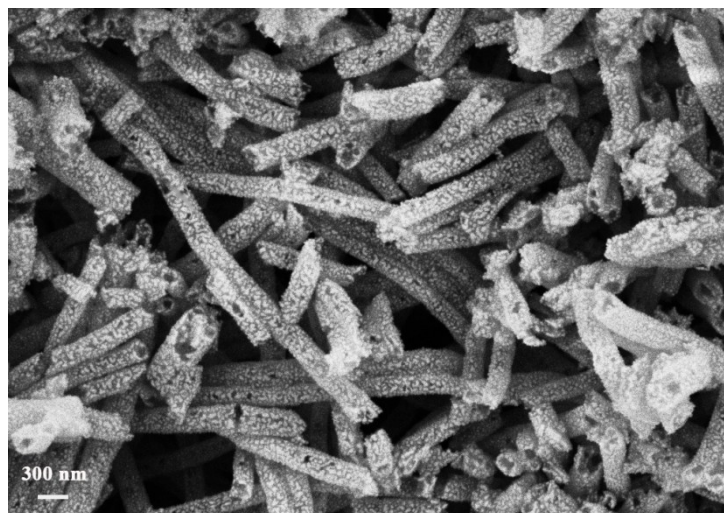
Figure S4. SEM image of the SnO 2 /SnS 2 nanotubes after NH 3 sensing test.
