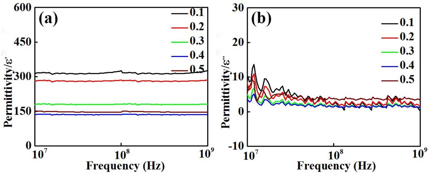
Fig. S4 (a) permittivity, (b) permitloss and (c) permitTan of BT-BFO-xLFO ( $x = 0.1-0.5$ ) ceramics sintered at 1300 °C
