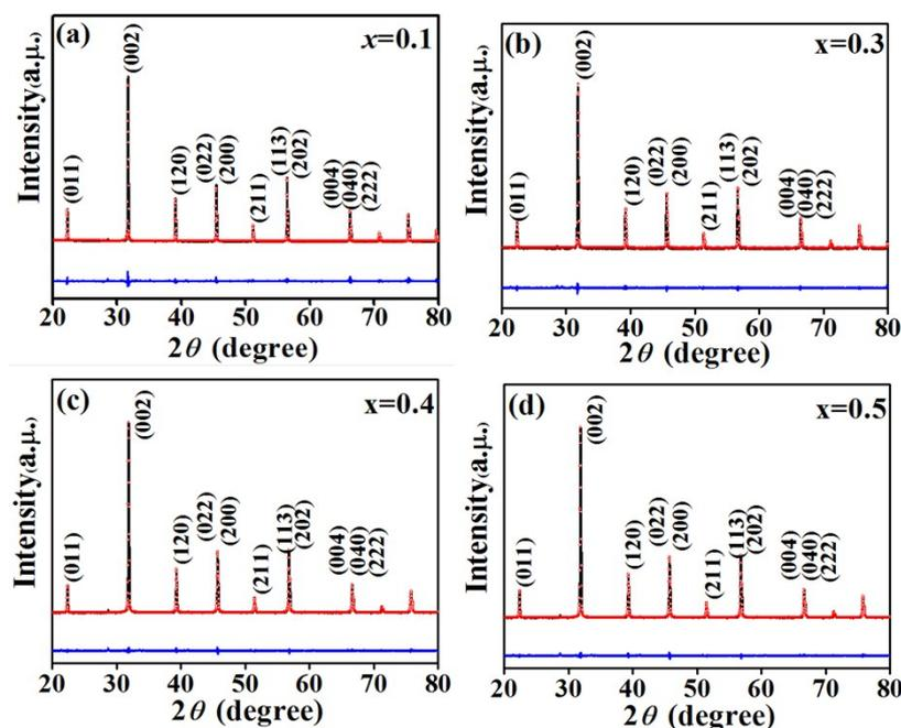
Fig. S1 XRD refinement of the BT-BFO-xLFO (x = 0.1, 0.3, 0.4 and 0.5)
