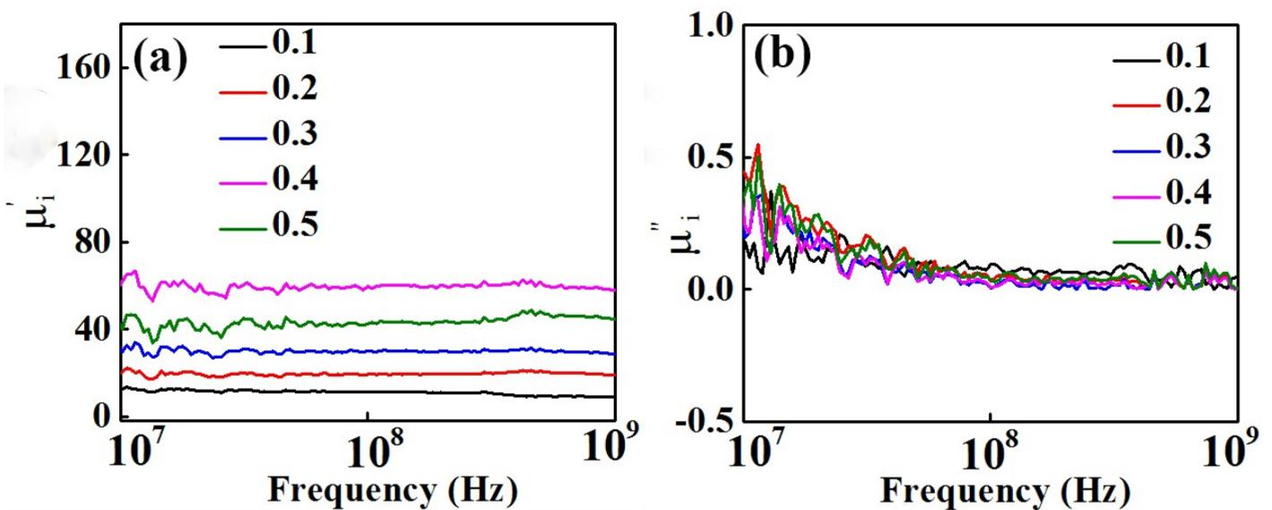
Fig. S5 (a)  $\mu_i'$  and (b)  $\mu_i''$  of BT-BFO-xLFO ( $x = 0.1-0.5$ ) ceramics sintered at 1300 °C
