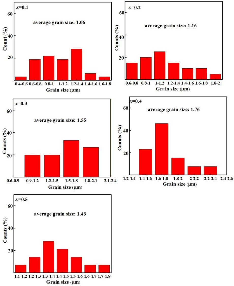
Fig. S2 Grain size distributions of the BT-BFO-xLFO (x = 0.1–0.5) ceramics sintered at 1300 °C
