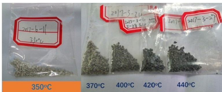
Fig. S5 The photos of the used catalyst with different reaction temperatures.
