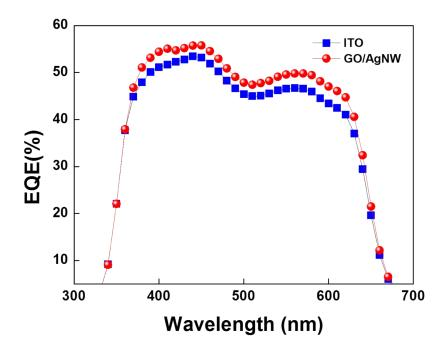
**SI 4.** EQE spectra of an OSC with the GO/Ag NW electrode and the reference device with the ITO electrode under AM 1.5 G illumination with 100 mW/cm<sup>2</sup> intensity.
