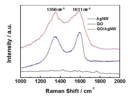
**SI 2.** Raman spectra before and after applying the GO coating to the AgNW film on the PET substrate.
