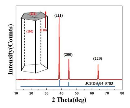
**SI 3.** X-ray diffraction (XRD) pattern of the synthesized AgNW and the standard powder pattern of Ag from JCPDS No. 04-0783.
