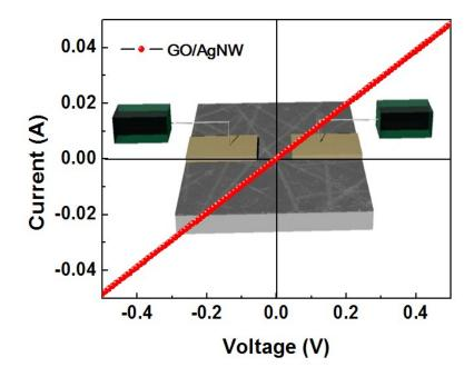
**SI 1.** Schematic diagram of the Au/GO/AgNW/PET device; the current between the two Au electrodes is a linear function of the applied voltage, which indicates excellent ohmic transport through the GO OCL.
