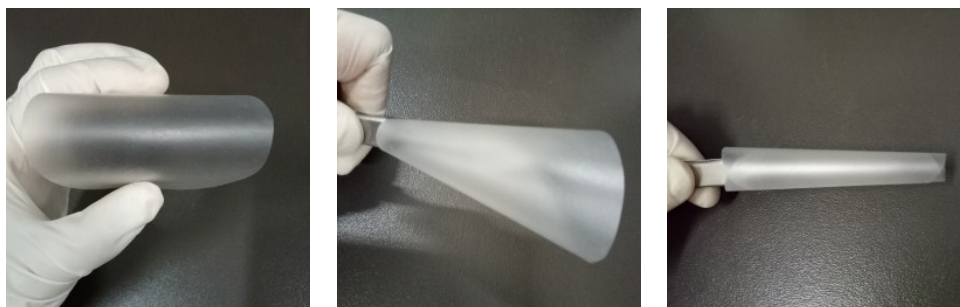
Fig. S3 Bending degree of acetylated NFC film (NFC: AA ratio was 1:3)
