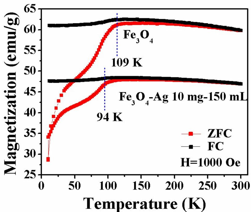
Fig. S7 ZFC and FC curves of pure  $\text{Fe}_3\text{O}_4$  and  $\text{Fe}_3\text{O}_4$ -Ag 10 mg-150 mL under an applied field of 1000 Oe.
