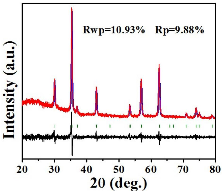
Fig. S1 Pawley refinement of the XRD pattern of the pure  $\text{Fe}_3\text{O}_4$ . Red dots, blue lines and olive bars represent the experimental data, the calculated data and the peak position of the sample, respectively. The bottom line in black shows the different experimental–calculated data.
