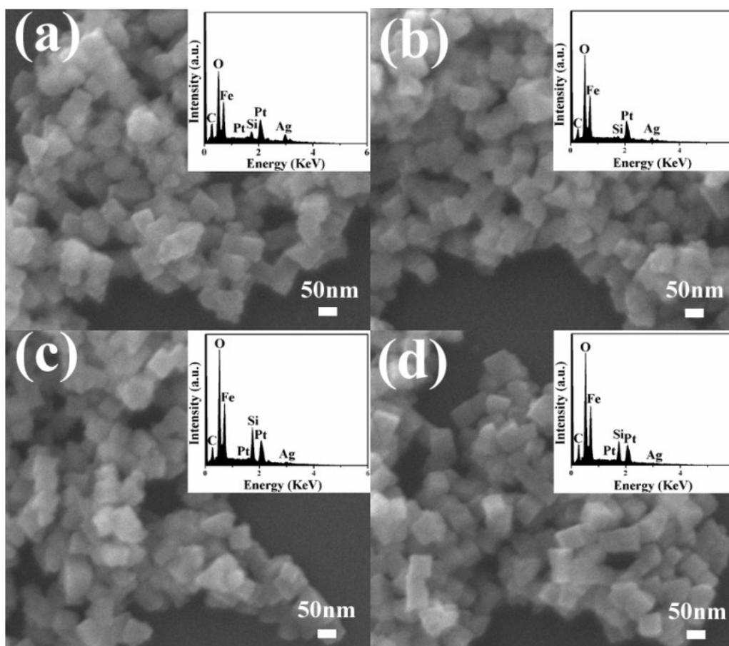
**Fig. S5** SEM images of Fe<sub>3</sub>O<sub>4</sub>-Ag 5 mg-30 mL (a), Fe<sub>3</sub>O<sub>4</sub>-Ag 10 mg-30 mL (b), Fe<sub>3</sub>O<sub>4</sub>-Ag 15 mg-30 mL (c) and Fe<sub>3</sub>O<sub>4</sub>-Ag 20 mg-30 mL (d). Insets are the corresponding energy-dispersive spectroscopy (EDS) spectra.
