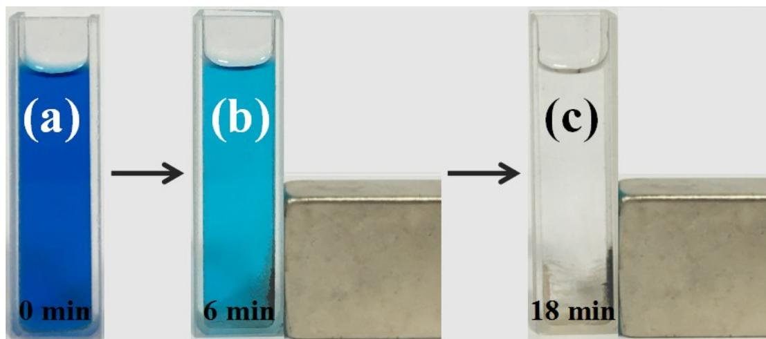
**Fig. S8** Color variation of MB over time catalyzed by Fe<sub>3</sub>O<sub>4</sub>-Ag 10 mg-100 mL.
