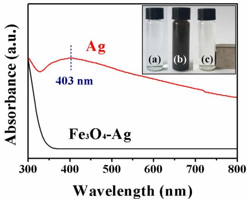
**Fig. S2** UV-vis spectra of the as-prepared colloidal Ag solution (red curve line) and the Ag solution after immobilization on the Fe<sub>3</sub>O<sub>4</sub>@PEI-DTC nanocrystals after the magnetic separation (black curve line). Inset shows the photographs of the colloidal Ag solution (a), reaction solution (b), and after magnetic separation (c).
