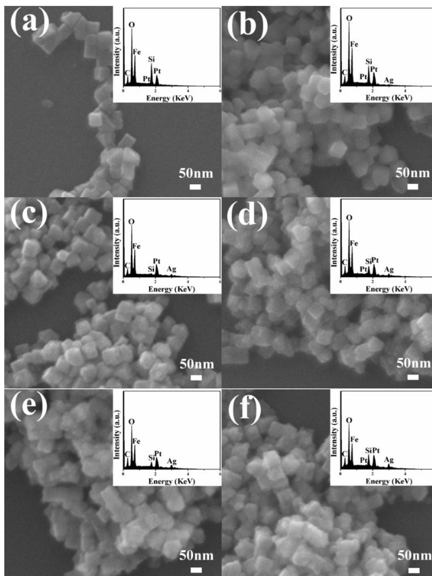
**Fig. S3** SEM images of  $\text{Fe}_3\text{O}_4$  (a),  $\text{Fe}_3\text{O}_4$ -Ag 10 mg-10 mL (b),  $\text{Fe}_3\text{O}_4$ -Ag 10 mg-30 mL (c),  $\text{Fe}_3\text{O}_4$ -Ag 10 mg-50 mL (d),  $\text{Fe}_3\text{O}_4$ -Ag 10 mg-100 mL (e) and  $\text{Fe}_3\text{O}_4$ -Ag 10 mg-150 mL (f). The insets are the corresponding energy-dispersive spectroscopy (EDS) spectra.
