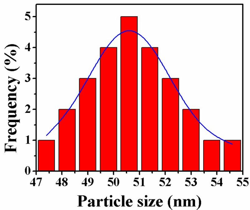
**Fig. S4** Histogram of pure Fe<sub>3</sub>O<sub>4</sub> nanocrystals from SEM image of Fig. S2 (a).
