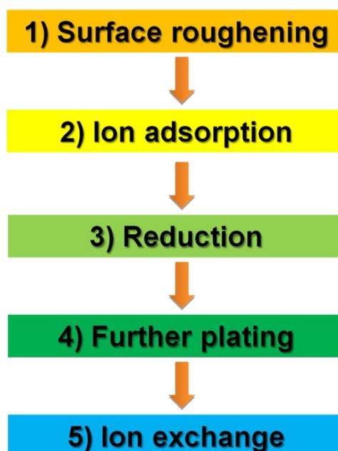
FIG. 1. The major steps of the preparation process for the IPMC.
