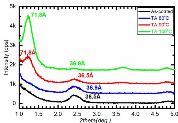
**Fig. S4** Thin film XRD pattern of Ph-(Tp)<sub>3</sub>-C18 before and after TA at different temperatures in the crystal state
