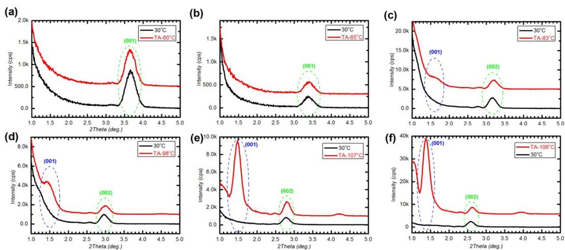
**Fig. S5** Thin film XRD patterns of (a) Ph-(Tp)<sub>3</sub>-C6, (b) Ph-(Tp)<sub>3</sub>-C8 at Cr1 phase and TA at a temperature near the transition point of Cr to SmE; thin film XRD patterns of (c) Ph-(Tp)<sub>3</sub>-C10, (d) Ph-(Tp)<sub>3</sub>-C12, (e) Ph-(Tp)<sub>3</sub>-C14, (f) Ph-(Tp)<sub>3</sub>-C16 before and after TA at Cr2 phase.
