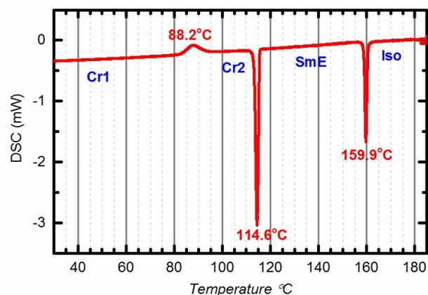
**Fig. S6** DSC of Ph-(Tp)<sub>3</sub>-C18 at 1°C min<sup>-1</sup> on 2<sup>nd</sup> heating run (the sample was firstly heated to Iso and then quenched by liquid N<sub>2</sub>)
