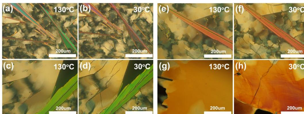
Fig. S2 POM textures of Ph-(Tp)<sub>3</sub>-C16 at 130°C (a), at 30°C (b); Ph-(Tp)<sub>3</sub>-C12 at 130°C (c), at 30°C (d); Ph-(Tp)<sub>3</sub>-C10 at 130°C (e), at 30°C (f); Ph-(Tp)<sub>3</sub>-C6 at 130°C (g), at 30°C (h).
