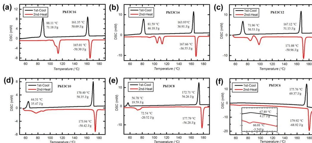
Fig. S1 DSC curves (10°C min<sup>-1</sup>) of Ph-(Tp)<sub>3</sub>-Cn (6, 8, 10, 12, 14, 16)
