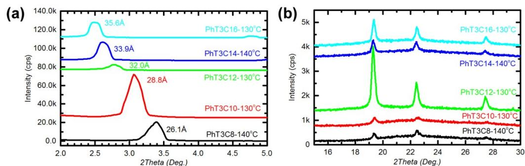
Fig. S3 Bulk film XRD patterns of Ph-(Tp)<sub>3</sub>-Cn (8, 10, 12, 14, 16) on heating at SmE phase.
