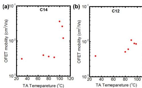
**Fig. S8** FET mobility of as a function of TA temperatures in Cr state (a)Ph-(Tp)<sub>3</sub>-C14 (b) Ph-(Tp)<sub>3</sub>-C12
