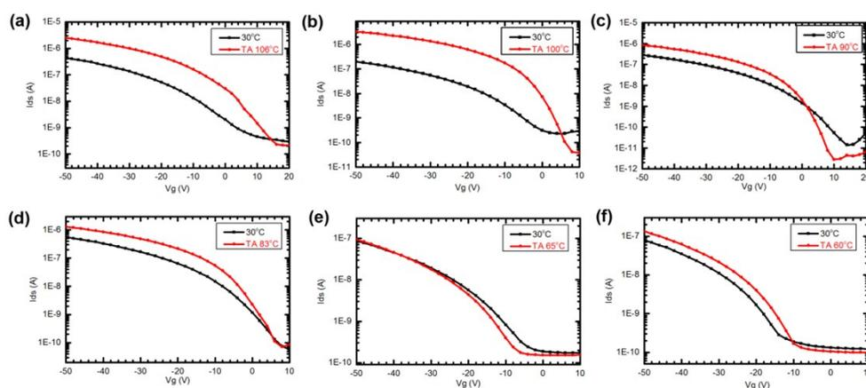
**Fig. S7** Transfer characteristics of (a) Ph-(Tp)<sub>3</sub>-C16, (b) Ph-(Tp)<sub>3</sub>-C14, (c) Ph-(Tp)<sub>3</sub>-C12, (d) Ph-(Tp)<sub>3</sub>-C10 before and after TA at Cr2 phase; (e) Ph-(Tp)<sub>3</sub>-C8, (f) Ph-(Tp)<sub>3</sub>-C6 at Cr1 phase and TA at a temperature near the transition point of Cr to SmE ( $V_{ds} = -50V$ ).
