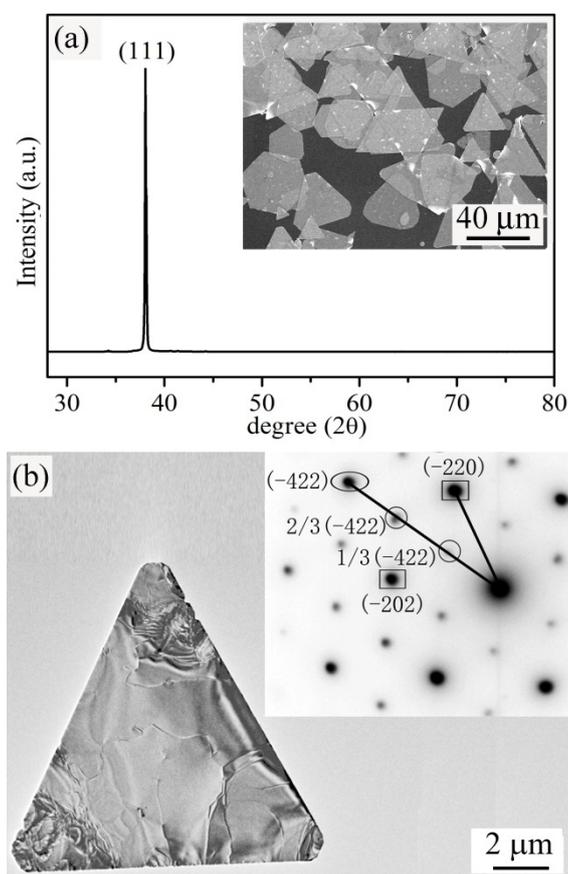
**Fig. S1.** (a) XRD pattern and FESEM image of Ag nanoflakes, (b) a typical TEM image of a triangle Ag nanoflakes and the corresponding SAED pattern.
