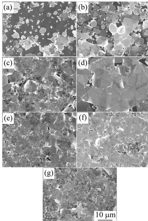
**Fig. S2.** FESEM images of Ag nanoflakes with PVP-K60 concentration of (a) 0.09, (b) 0.18, (c) 0.27, (d) 0.36, (e) 0.45, (f) 0.54 and (g) 0.63 M.
