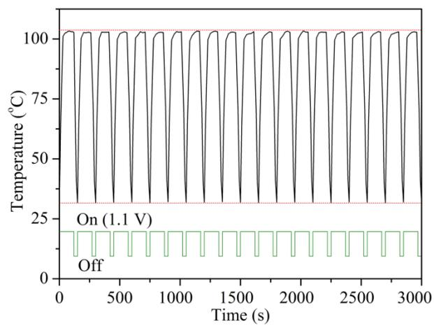
**Fig. S6.** Temperature profile of Ag nanoflakes heater within 20 cycles at an applied voltage of 1.1 V.
