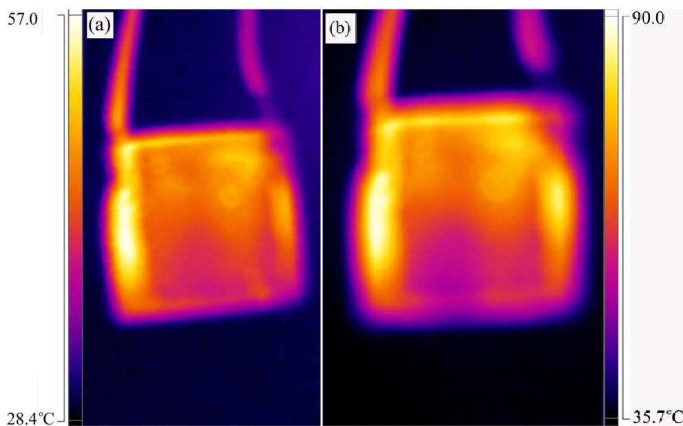
**Fig. S5.** Infrared photographs of Ag nanoflakes film heater at constant input voltage of (a) 0.5 and (b) 0.8 V with the surface temperature of 43.1 and 62.8 °C, respectively.
