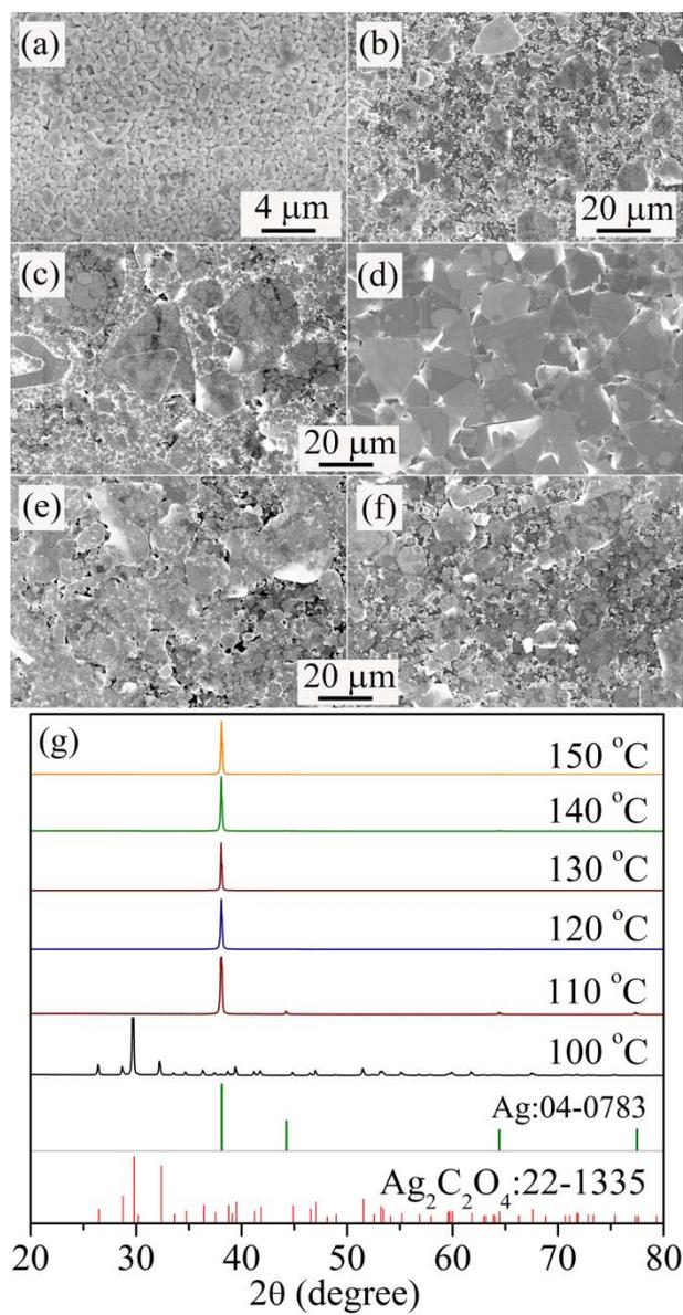
**Fig. S3.** FESEM images of Ag nanoflakes at reaction temperature of (a) 100, (b) 110, (c) 120, (d) 130, (e) 140, and (f) 150 °C. (g) The corresponding XRD spectra of the products at different temperatures.
